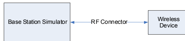
Figure 8-2 Power Measurement Setup
