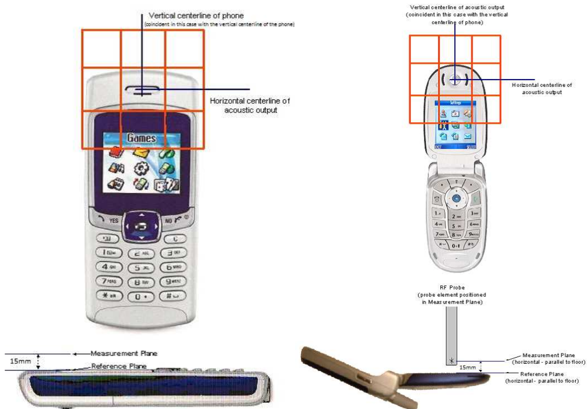
Figure 5.1 Wireless Device and Measurement Plane
