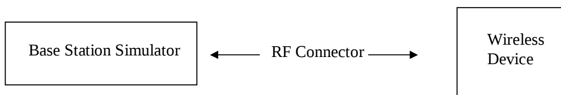
Figure 9-1 Power Measurement Setup
