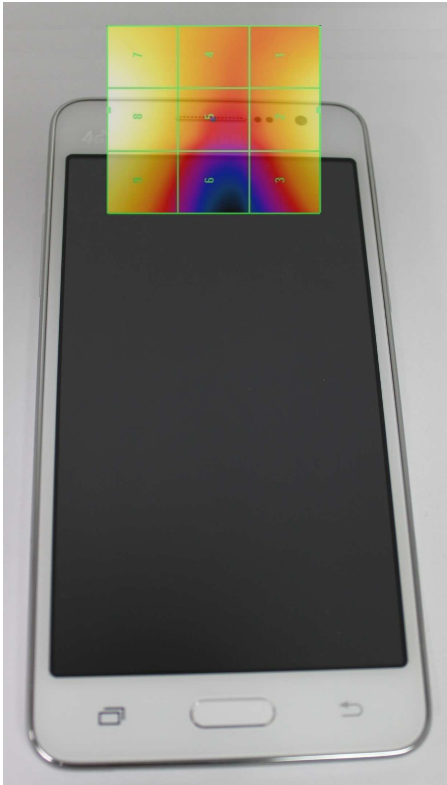
Scan Overlay with actual device(E-Field)
