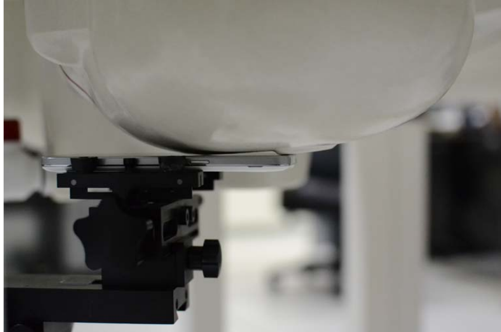
SAR Test Setup Photo 3 – Left Cheek
