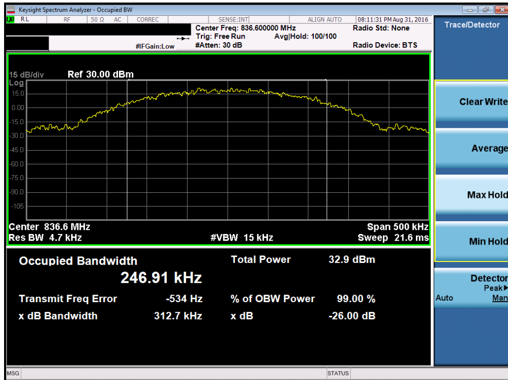
Plot 7-2. Occupied Bandwidth Plot (EDGE850 Mode – Ch. 190)
