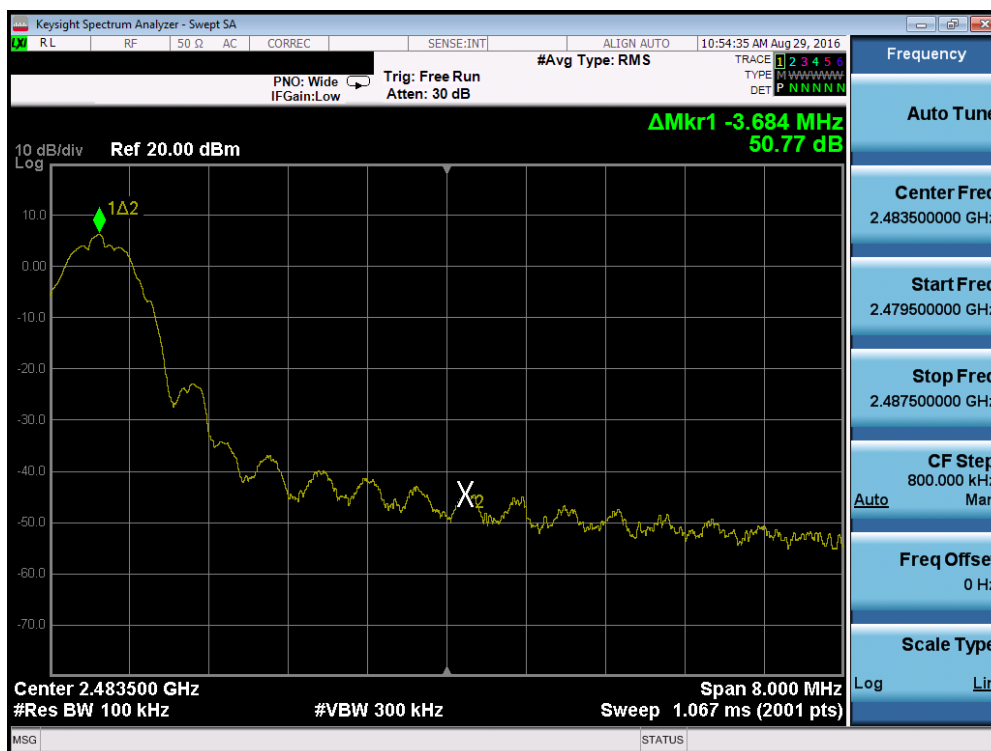
Plot 7-11. Band Edge Plot (Bluetooth (LE) – Ch. 39)
