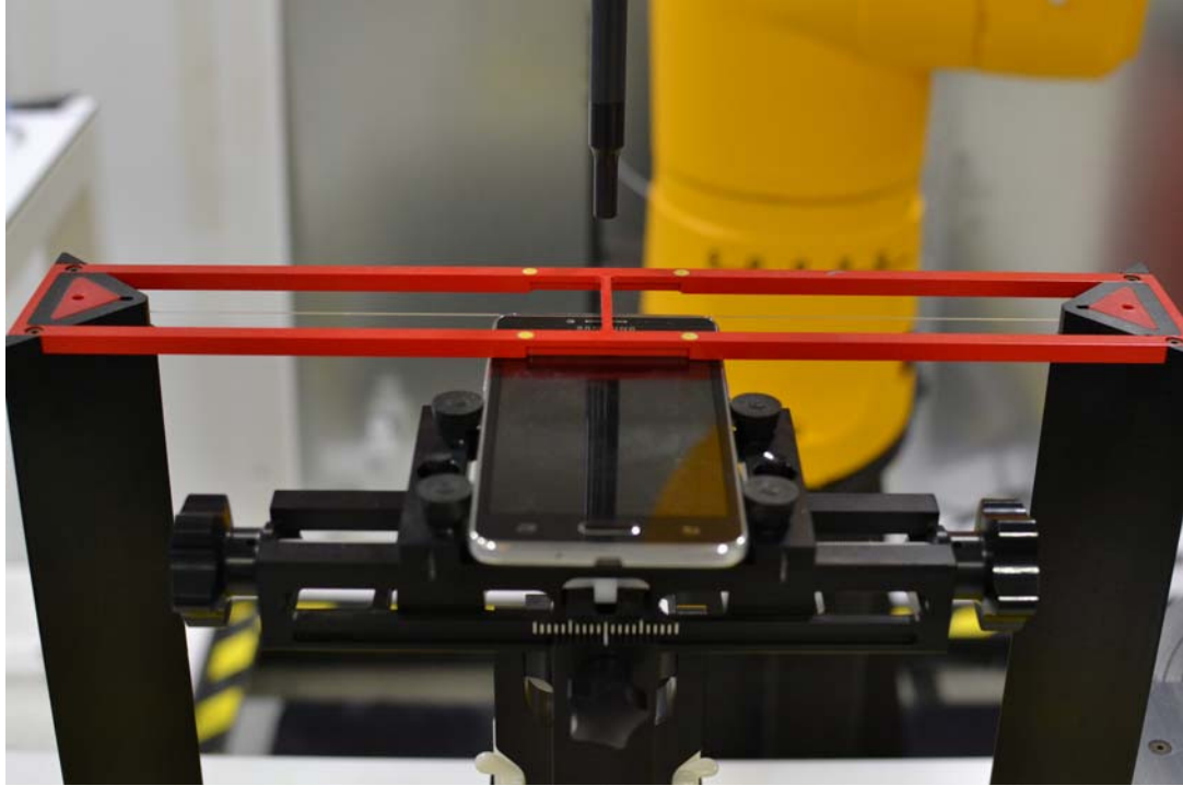
Figure 17-1 Ear Reference Point HAC Phantom Alignment
