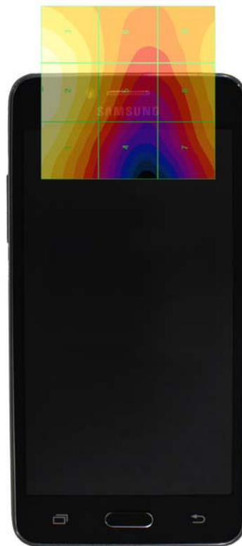
Figure 17-4 E-Field WD Scan overlay
