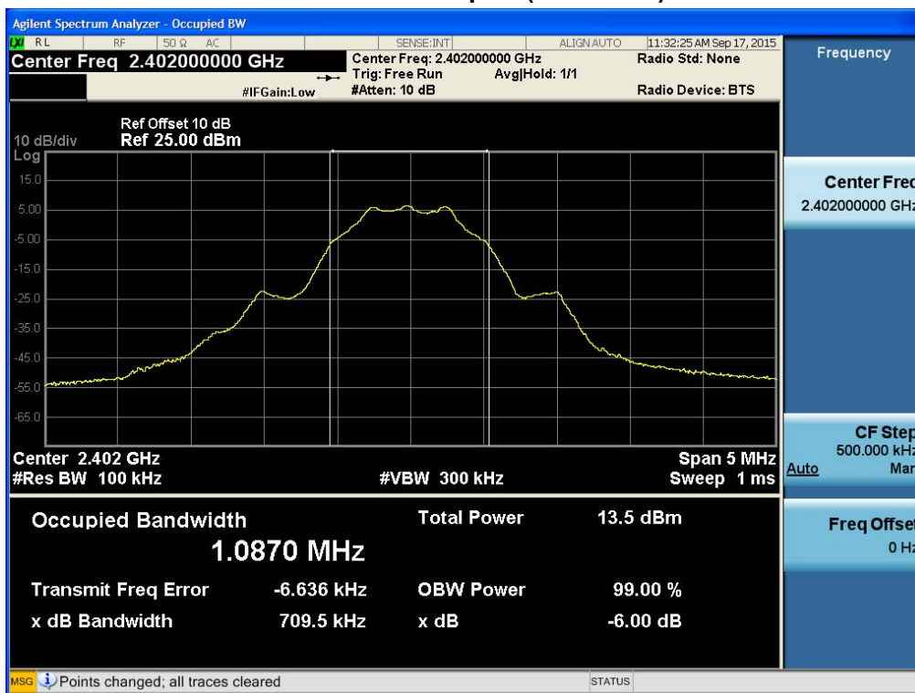
6dB Bandwidth plot (Low-CH 0)
