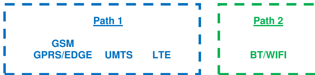
Figure 1-1 Simultaneous Transmission Paths
