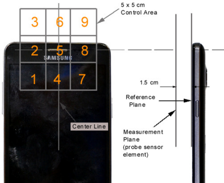
Figure 18-3 5x5 Scan grid above WD
