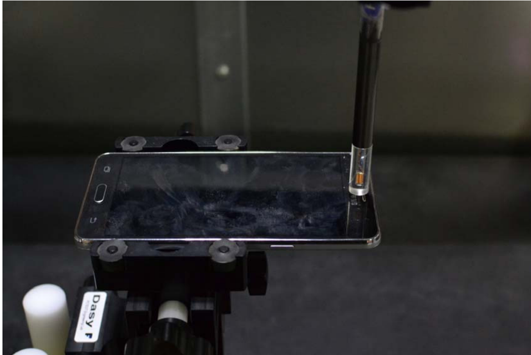
Figure 15-1 Test Setup for Wireless Device
