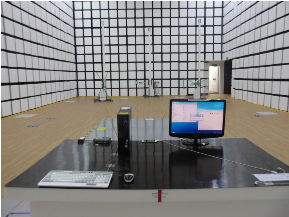
[ Radiated Disturbance for Below 1 GHz – Front ]
