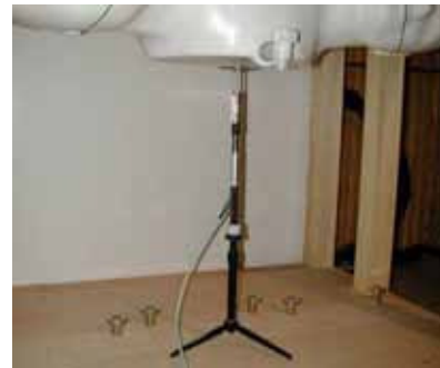
Figure 10-2 System Verification Setup Photo
