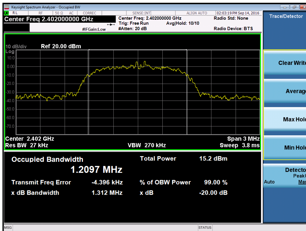
Plot 7-7. 20dB Bandwidth Plot (Bluetooth, 3Mbps – Ch. 0)
