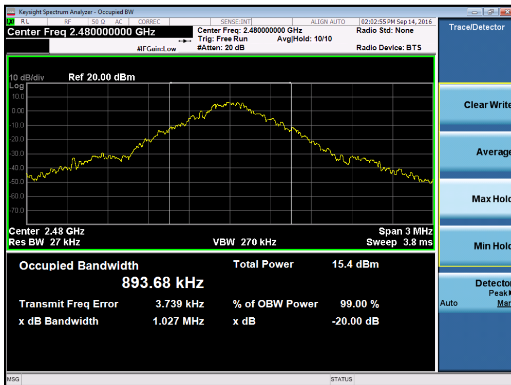
Plot 7-3. 20dB Bandwidth Plot (Bluetooth, 1Mbps – Ch. 78)
