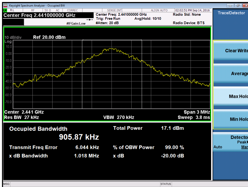
Plot 7-2. 20dB Bandwidth Plot (Bluetooth, 1Mbps – Ch. 39)
