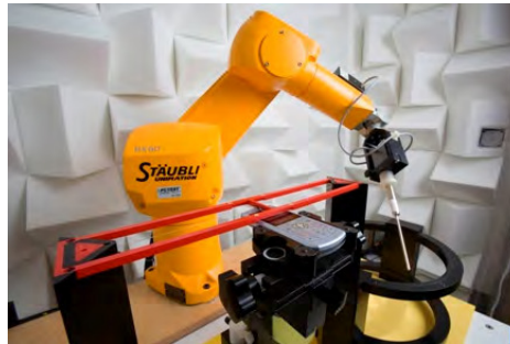
Figure 4-3 SPEAG Robotic System
