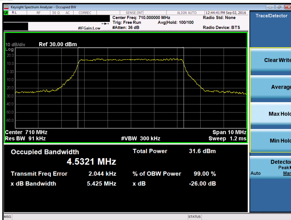
Plot 7-1. Occupied Bandwidth Plot (Band 17 – 5.0MHz QPSK – RB Size 25)
