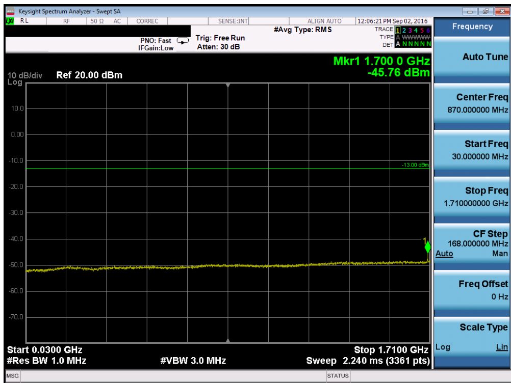
Plot 7-58. Conducted Spurious Plot (Band 4 – 15.0MHz QPSK – RB Size 1, RB Offset 0 – Mid Channel)
