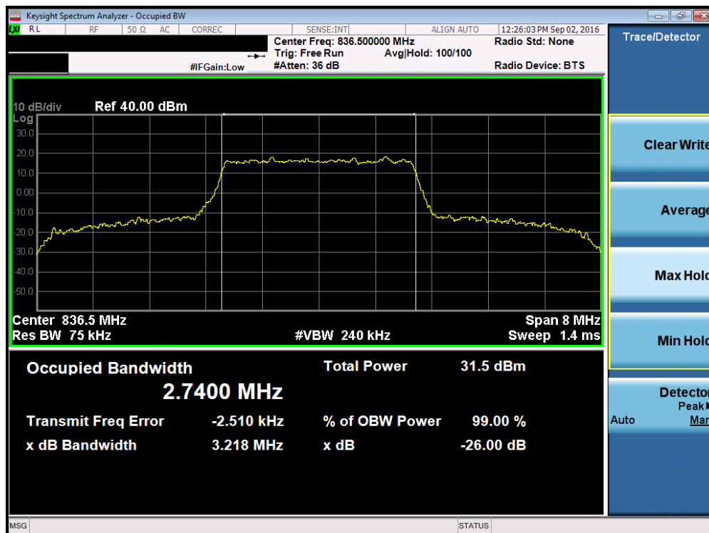
Plot 7-8. Occupied Bandwidth Plot (Band 5 – 3.0MHz 16-QAM – RB Size 15)
