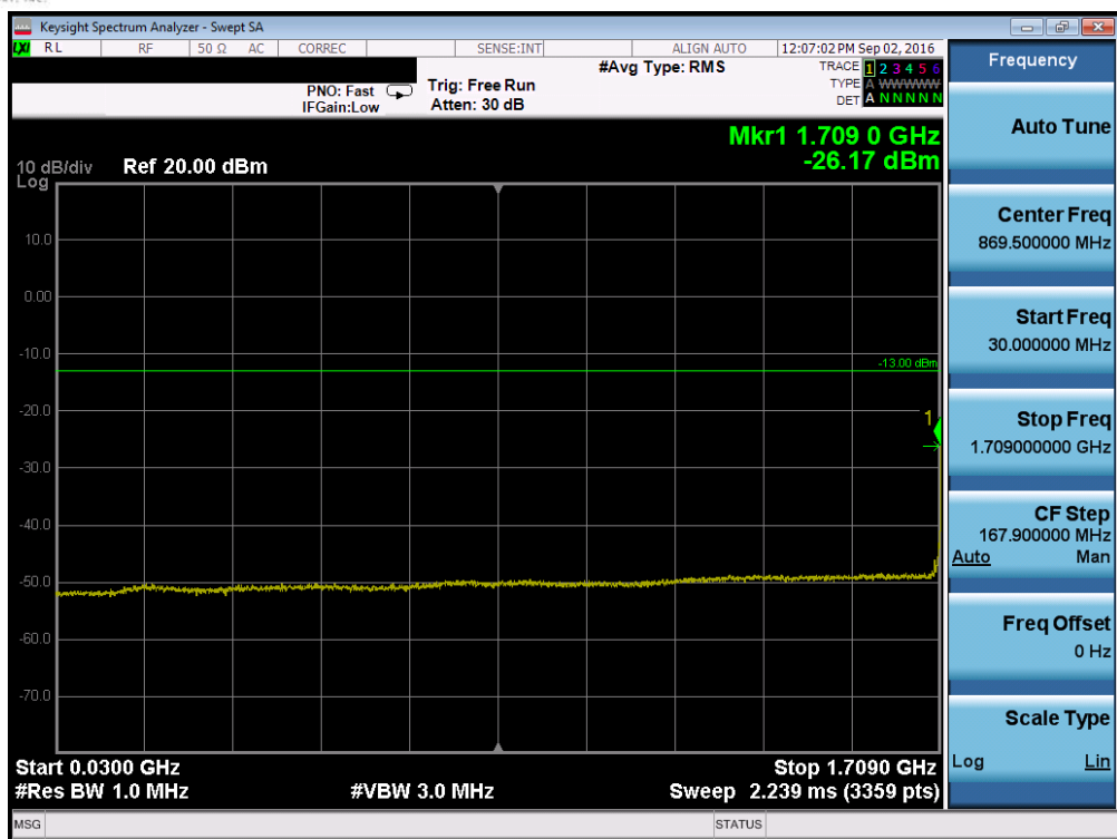
Plot 7-55. Conducted Spurious Plot (Band 4 – 15.0MHz QPSK – RB Size 1, RB Offset 0 – Low Channel)
