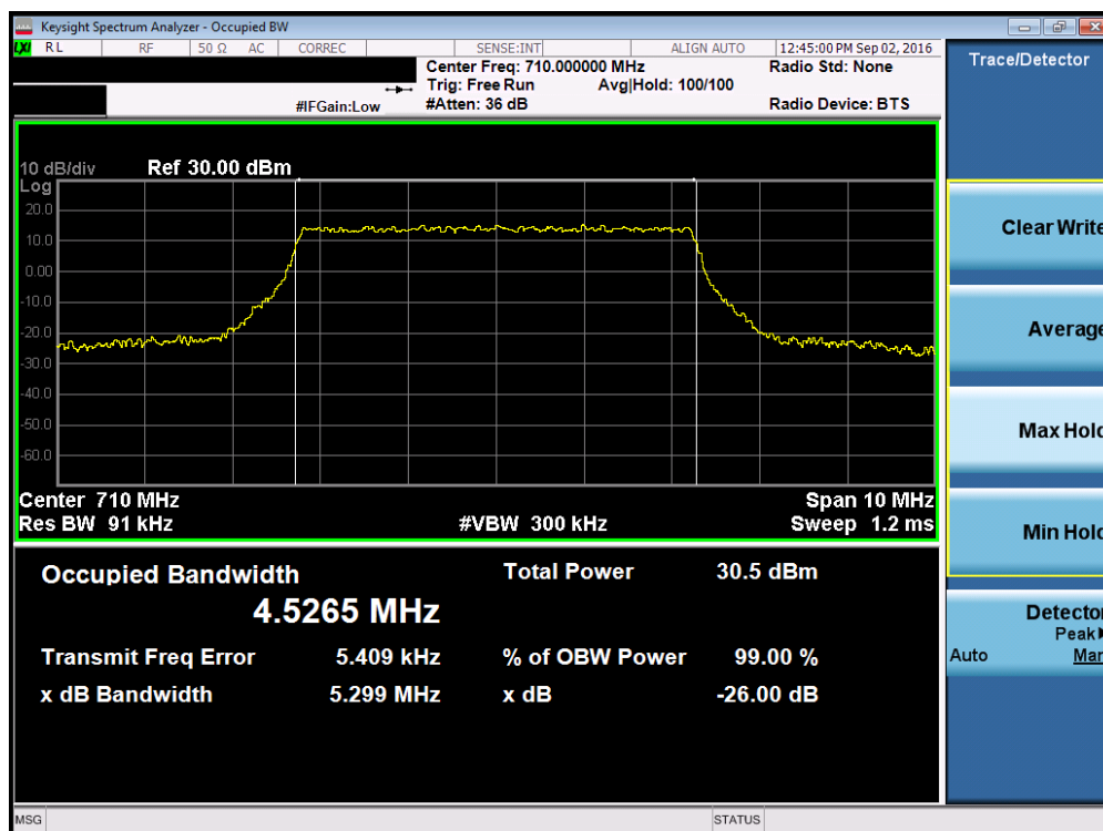
Plot 7-2. Occupied Bandwidth Plot (Band 17 – 5.0MHz 16-QAM – RB Size 25)
