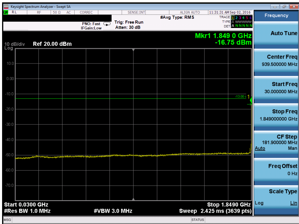
Plot 7-64. Conducted Spurious Plot (Band 2 – 10.0MHz QPSK – RB Size 1, RB Offset 0– Low Channel)
