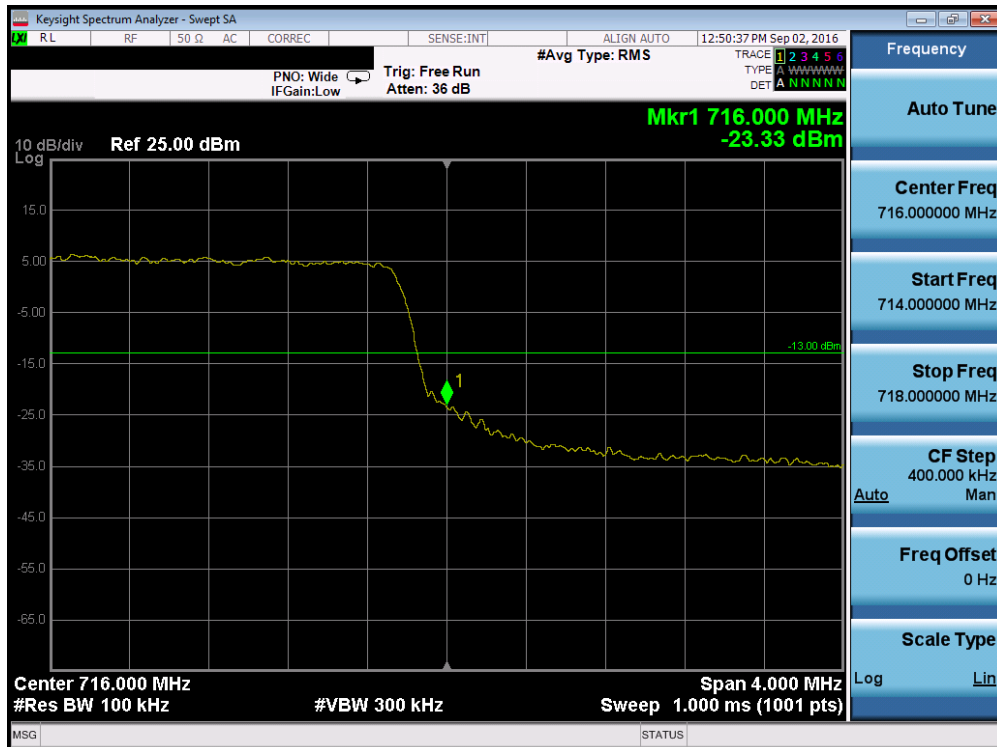
Plot 7-74. Upper Band Edge Plot (Band 17 - 5.0MHz QPSK - RB Size 25)
