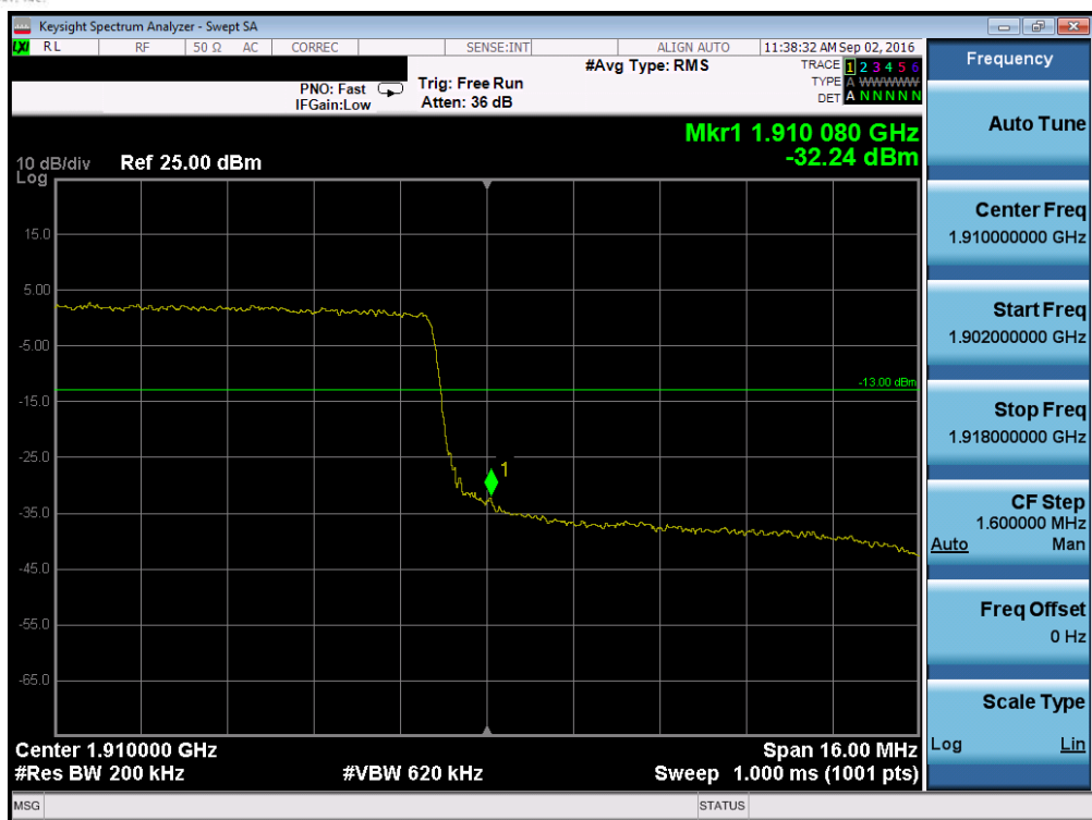
Plot 7-133. Upper Band Edge Plot (Band 2 – 20.0MHz QPSK – RB Size 100)
