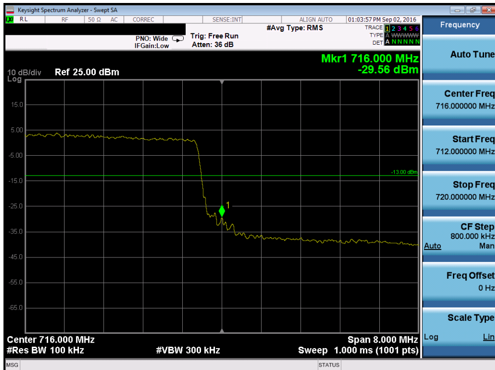
Plot 7-76. Upper Band Edge Plot (Band 17 – 10.0MHz QPSK – RB Size 50)
