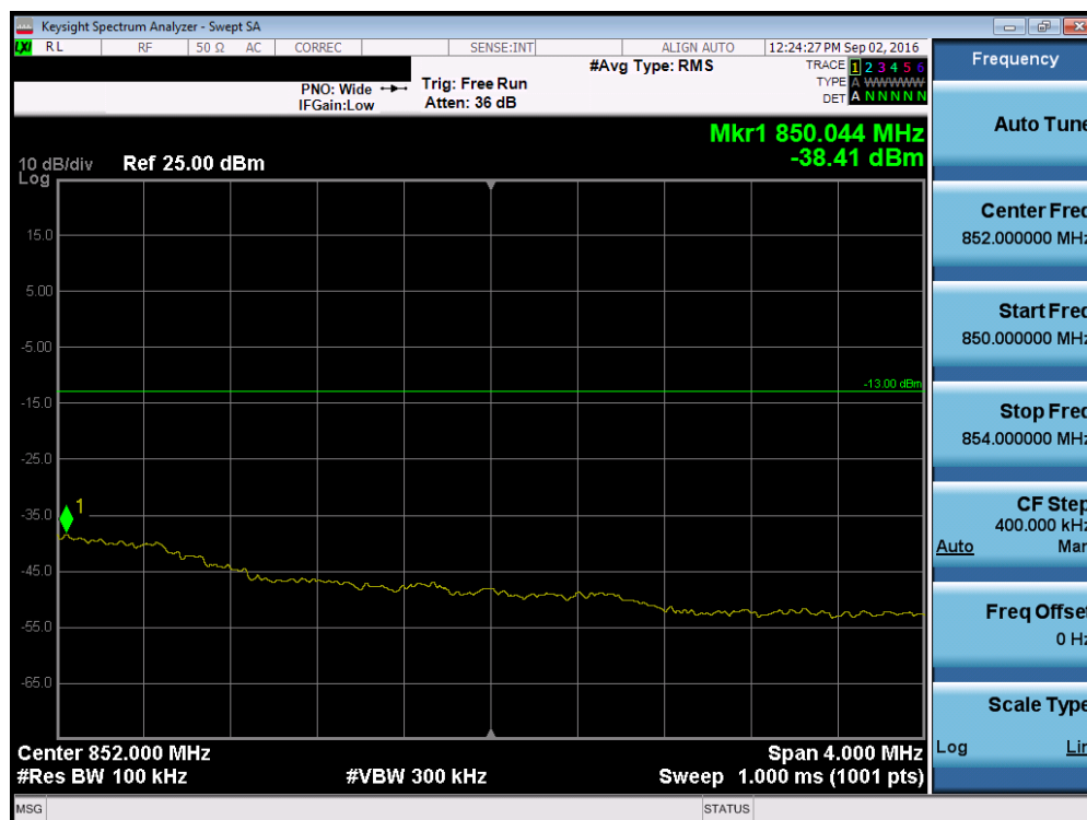
Plot 7-80. Upper Extended Band Edge Plot (Band 5 – 1.4MHz QPSK – RB Size 6)
