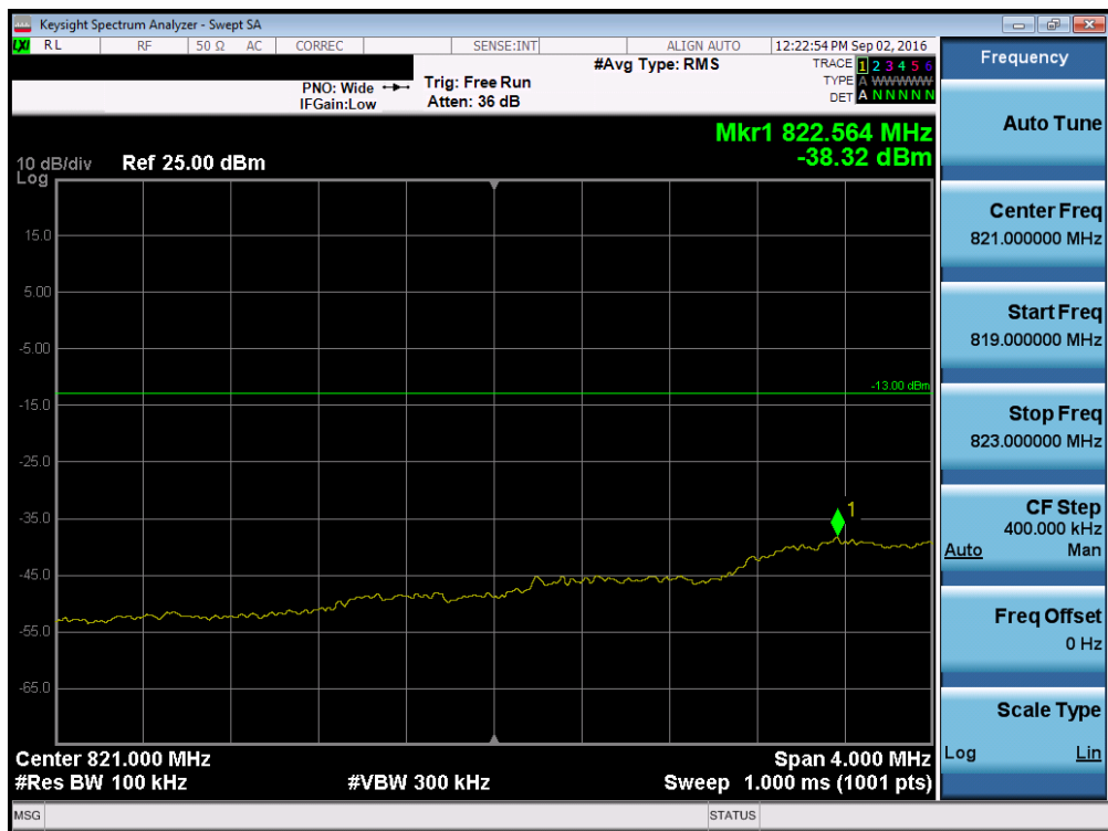
Plot 7-78. Lower Extended Band Edge Plot (Band 5 – 1.4MHz QPSK – RB Size 6)
