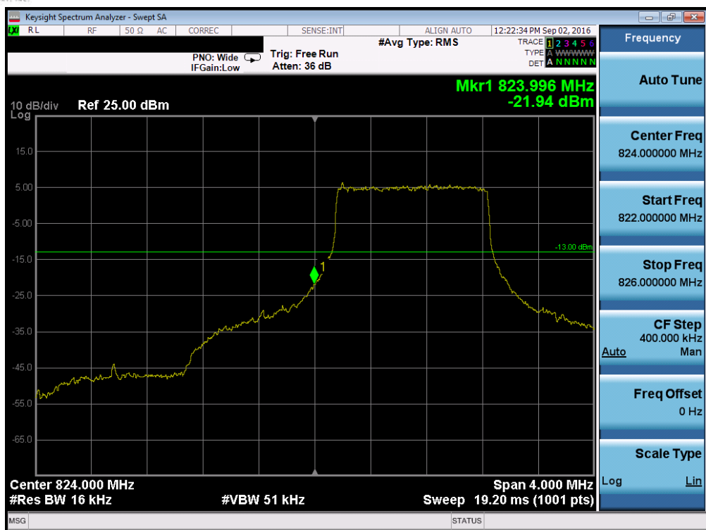
Plot 7-77. Lower Band Edge Plot (Band 5 – 1.4MHz QPSK – RB Size 6)
