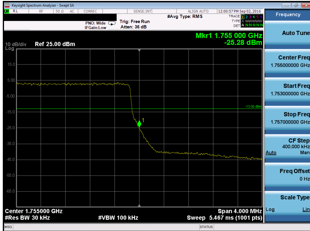
Plot 7-93. Upper Band Edge Plot (Band 4 – 3.0MHz QPSK – RB Size 15)
