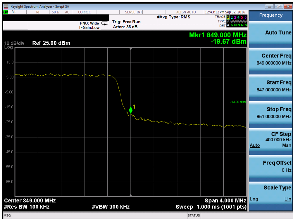
Plot 7-84. Upper Band Edge Plot (Band 5 – 5.0MHz QPSK – RB Size 25)
