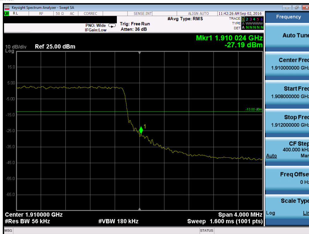
Plot 7-121. Upper Band Edge Plot (Band 2 – 5.0MHz QPSK – RB Size 25)
