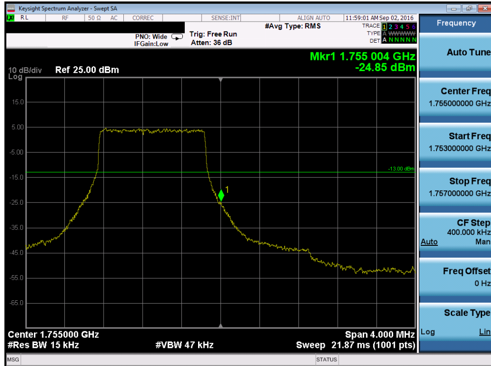
Plot 7-89. Upper Band Edge Plot (Band 4 – 1.4MHz QPSK – RB Size 6)
