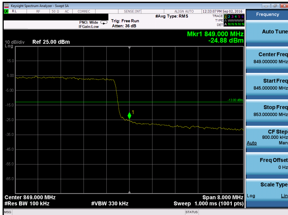
Plot 7-86. Upper Band Edge Plot (Band 5 - 10.0MHz QPSK - RB Size 50)
