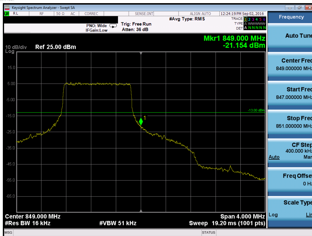
Plot 7-79. Upper Band Edge Plot (Band 5 – 1.4MHz QPSK – RB Size 6)
