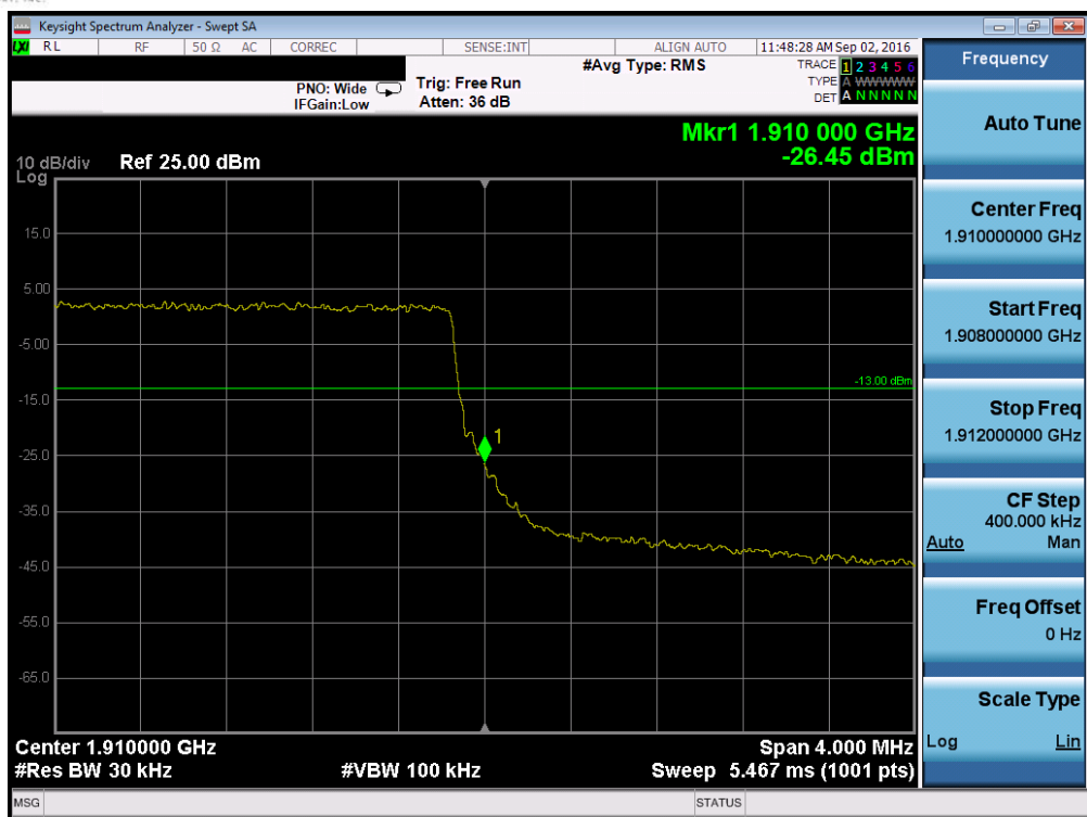
Plot 7-117. Upper Band Edge Plot (Band 2 – 3.0MHz QPSK – RB Size 15)
