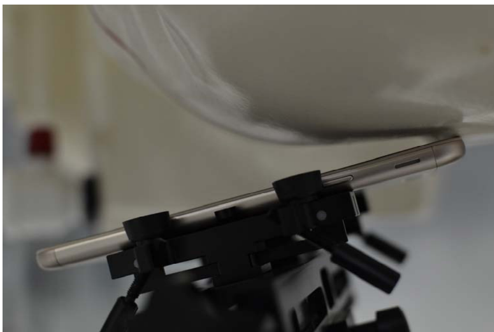
SAR Test Setup Photo 4 – Left Tilt
