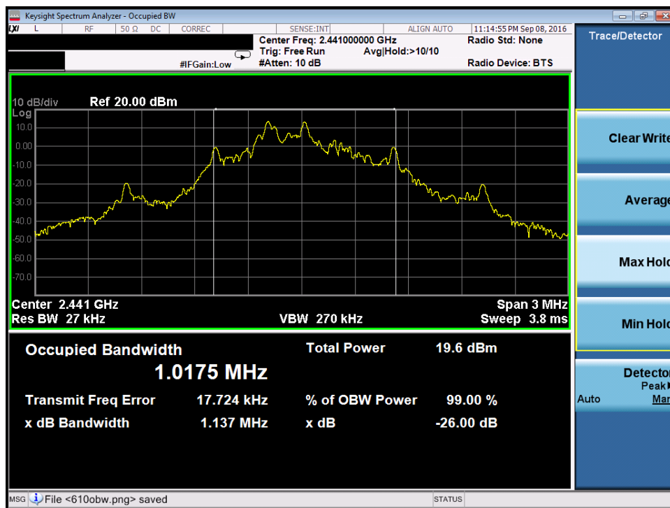
Plot 7-1. Occupied Bandwidth Plot (ANT+ – Ch. 39)
