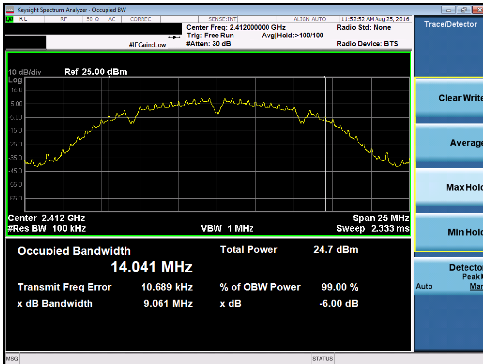
Plot 7-1. 6dB Bandwidth Plot (802.11b – Ch. 1)
