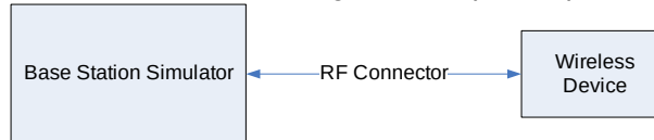
Figure 8-2 Power Measurement Setup
