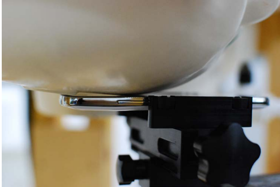
SAR Test Setup Photo 1 – Right Cheek
