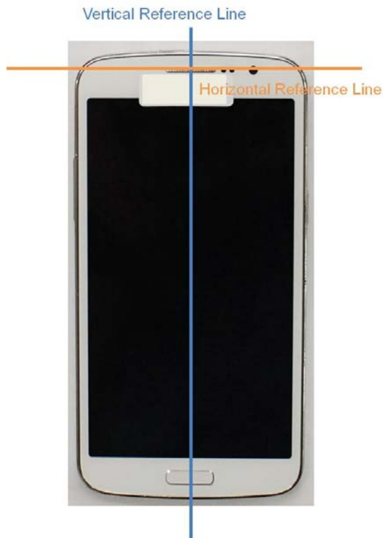
SAR Test Setup Photo 10 – Horizontal and Vertical Reference Lines
