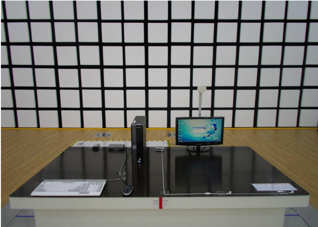
[ Radiated Disturbance for Below 1 GHz – Front ]
