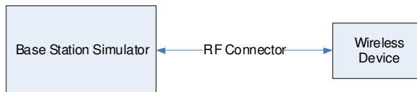
Figure 8-1 Power Measurement Setup
