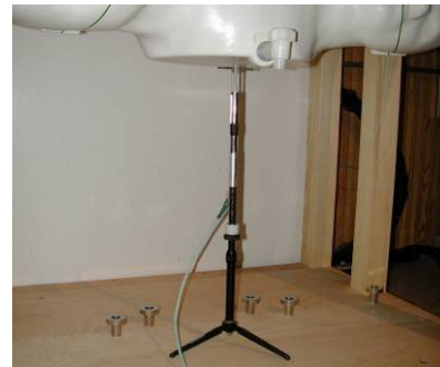
Figure 10-2 System Verification Setup Photo
