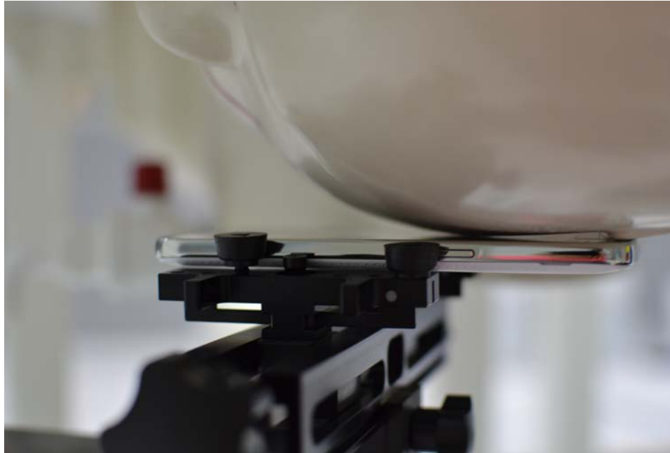
SAR Test Setup Photo 3 – Left Cheek
