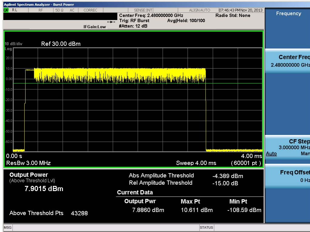
Plot 6-24. Average Conducted Power (2Mbps – Ch. 78)
