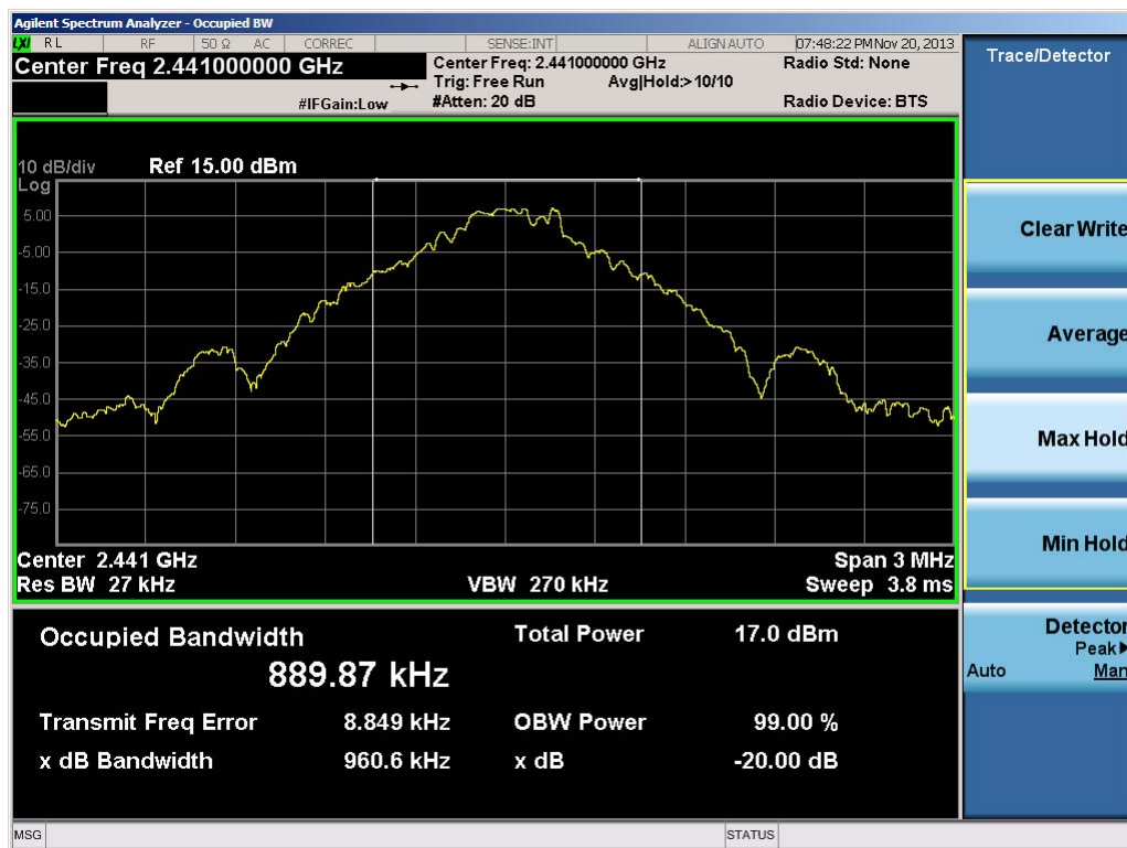
Plot 6-2. 20dB Bandwidth Plot (Bluetooth, 1Mbps – Ch. 39)
