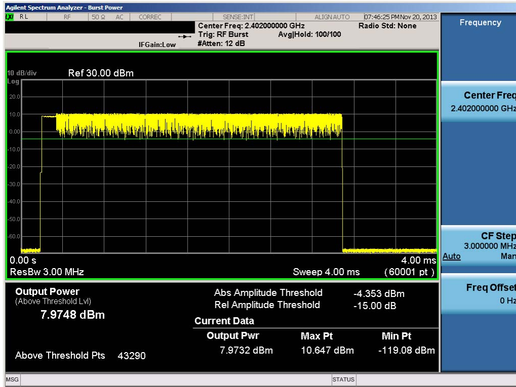
Plot 6-22. Average Conducted Power (2Mbps – Ch. 0)
