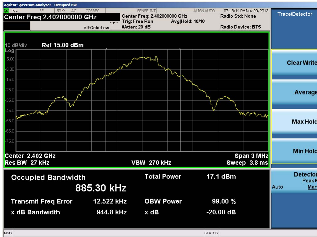
Plot 6-1. 20dB Bandwidth Plot (Bluetooth, 1Mbps – Ch. 0)
