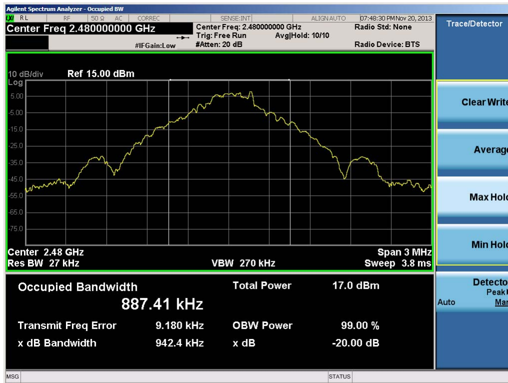
Plot 6-3. 20dB Bandwidth Plot (Bluetooth, 1Mbps – Ch. 78)
