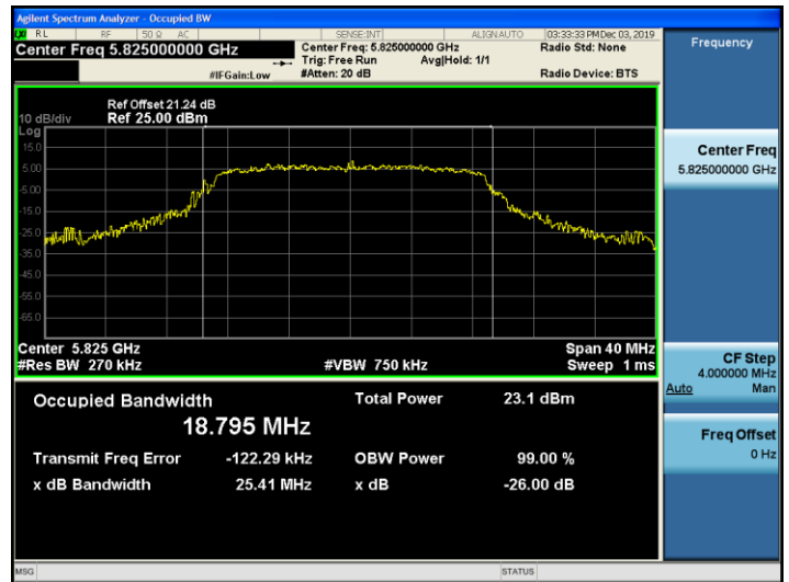
802.11n_HT20 UNII 3 BAND 26dB Bandwidth(CH 165)
