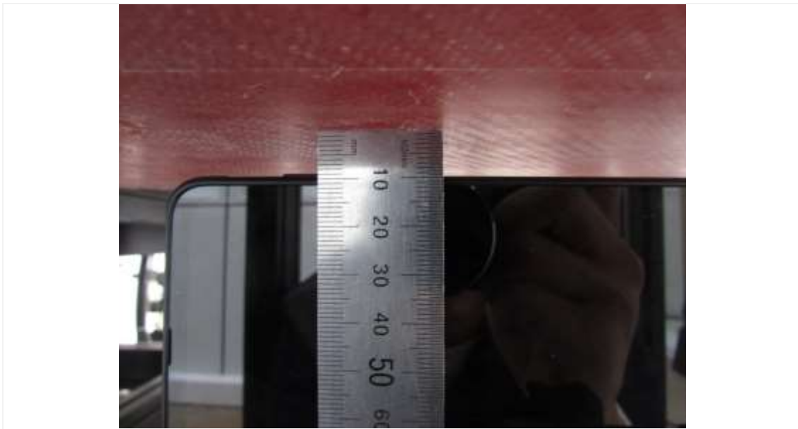
Distance of 10 mm from the EUT
