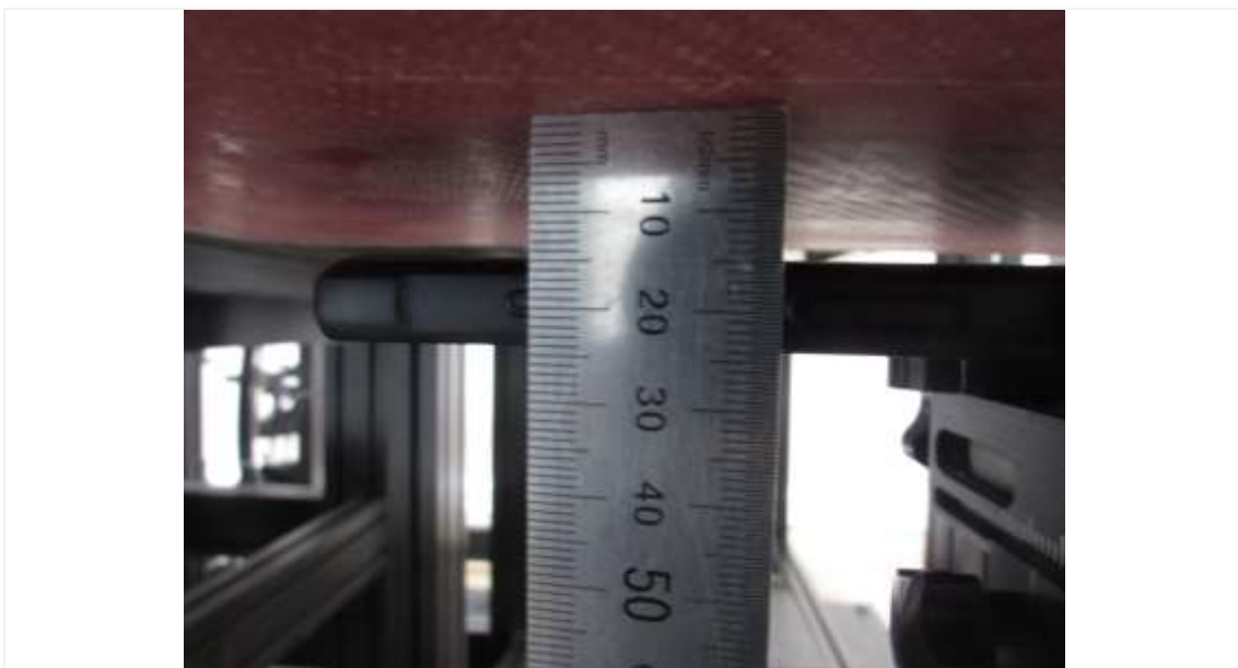
Distance of 15 mm from the EUT
