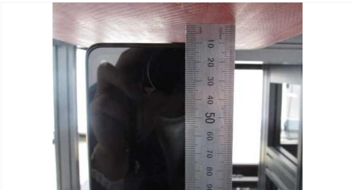
Distance of 10 mm from the EUT
