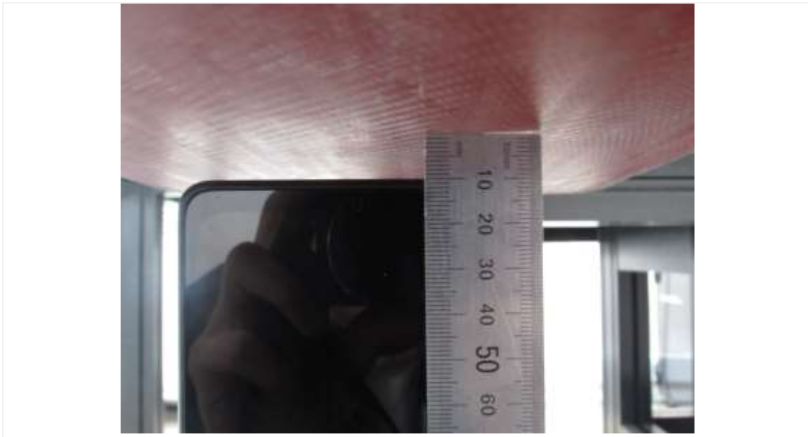
Distance of 10 mm from the EUT
