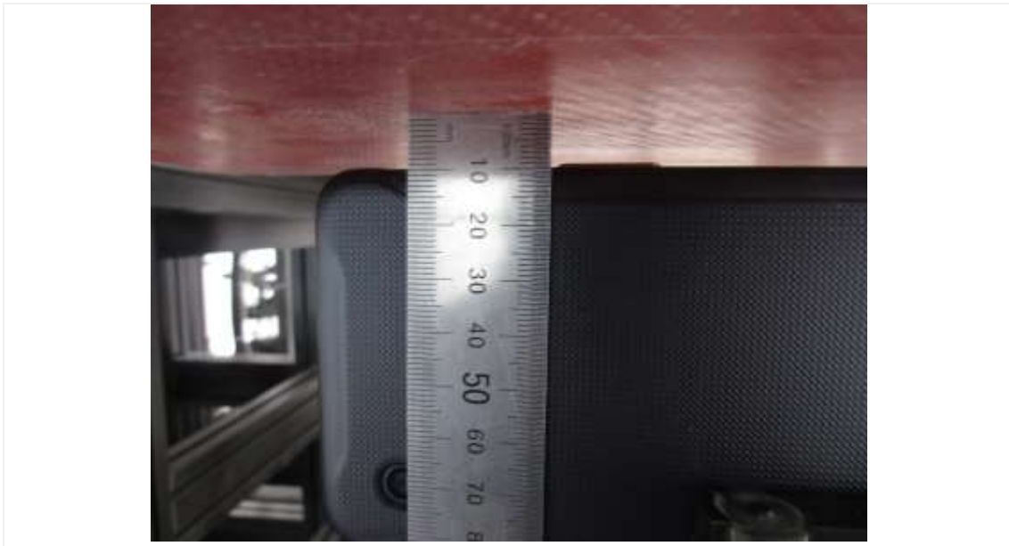
Distance of 10 mm from the EUT
