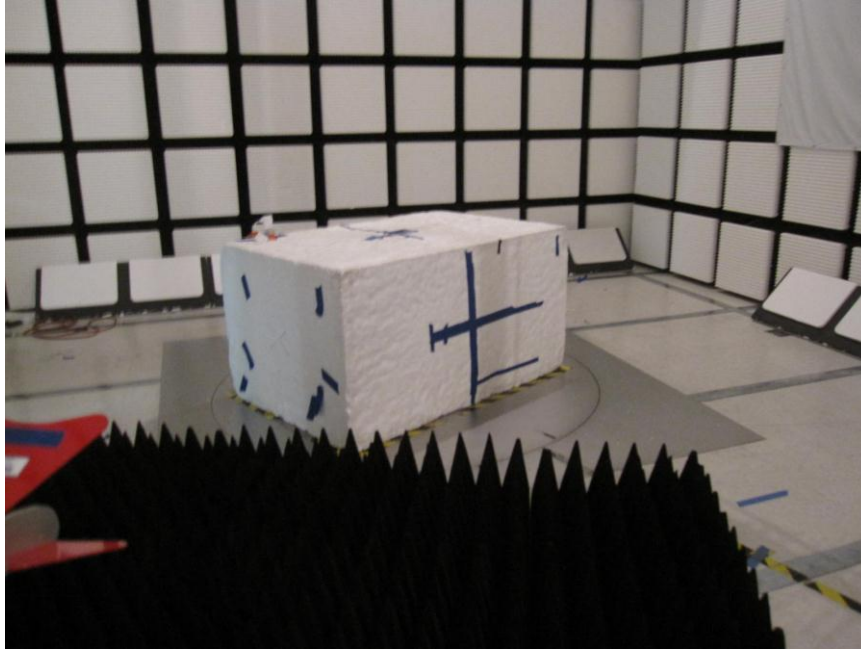
RADIATED FRONT PHOTO (ABOVE 1 GHz)
