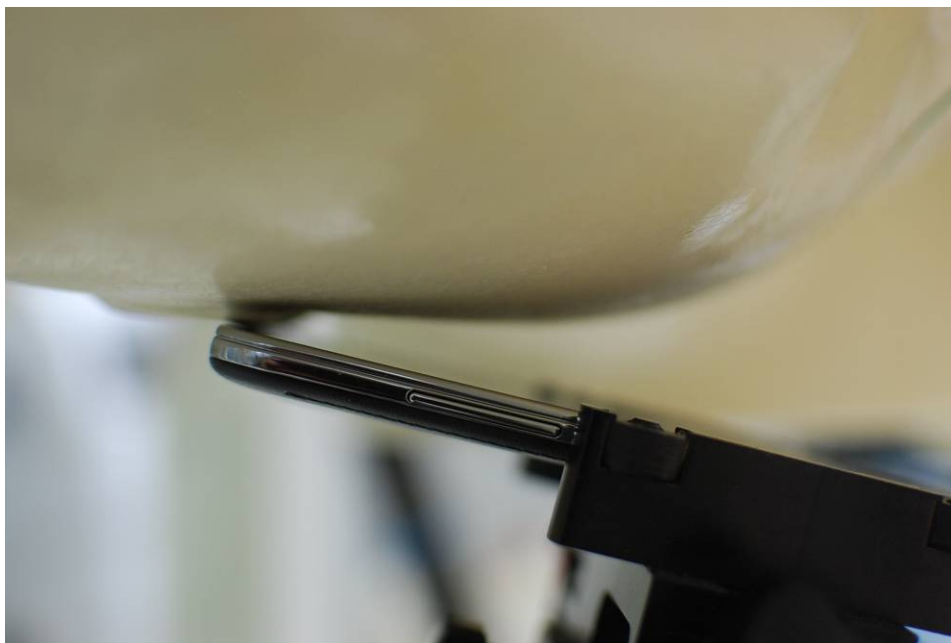
SAR Test Setup Photo 2 – Right Tilt
