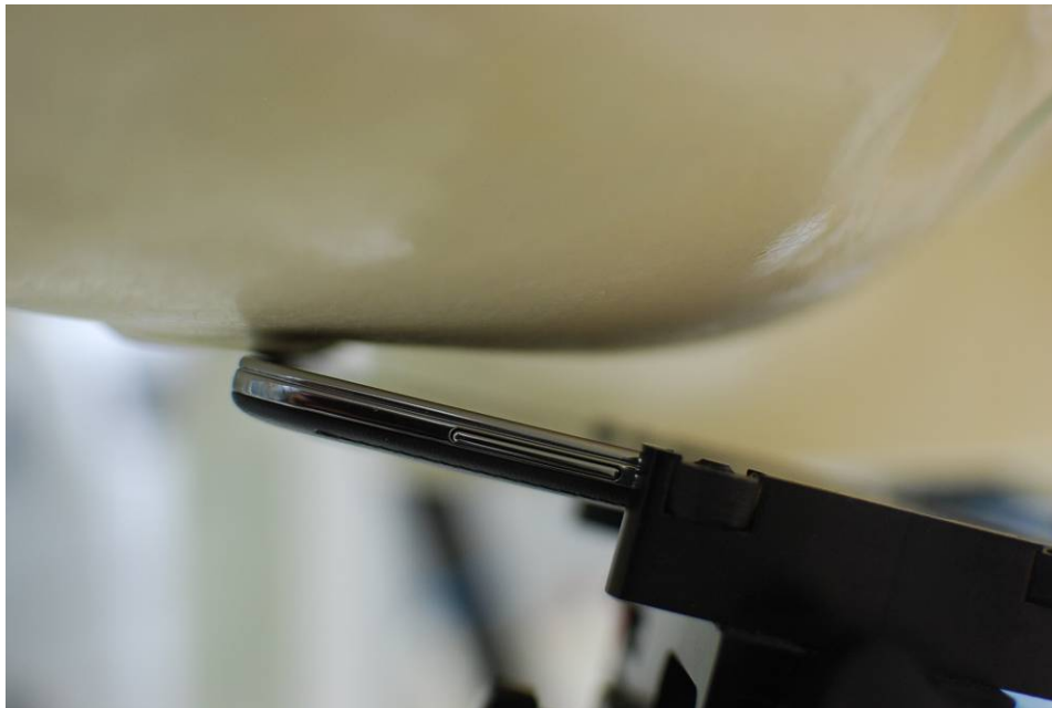
SAR Test Setup Photo 2 – Right Tilt
