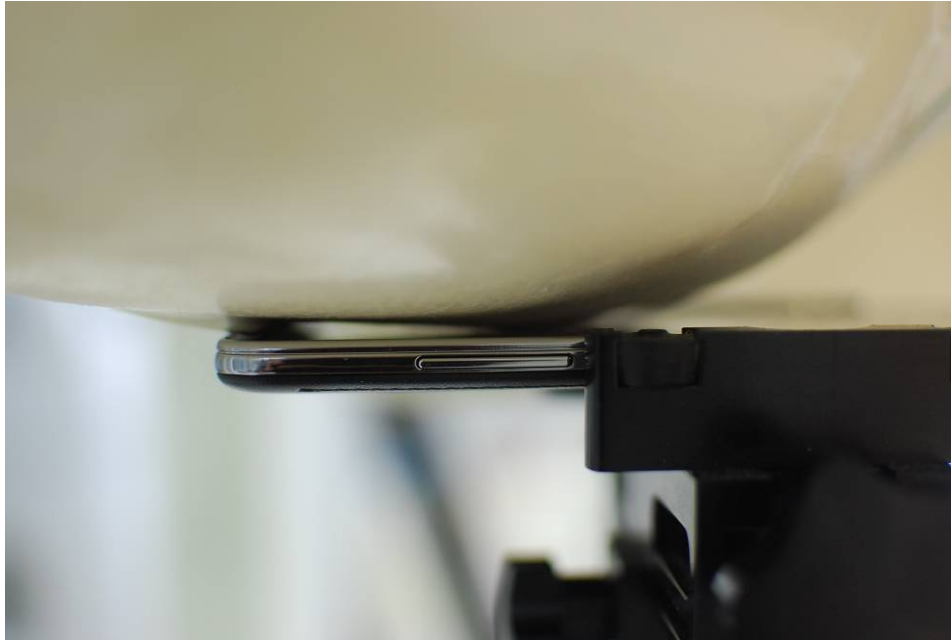
SAR Test Setup Photo 1 – Right Cheek
