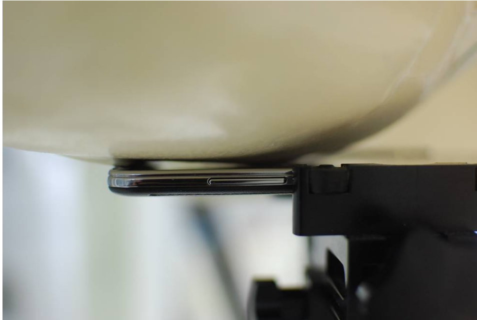
SAR Test Setup Photo 1 – Right Cheek
