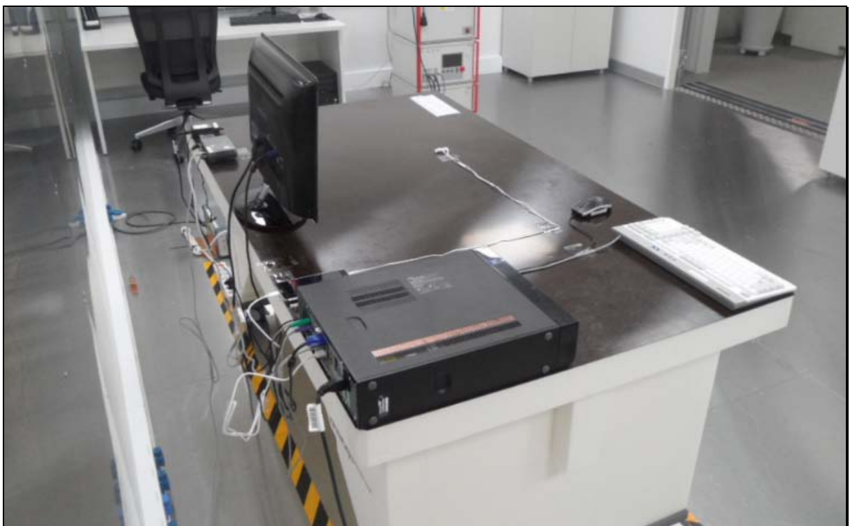
[ Conducted Disturbance – Rear ]
