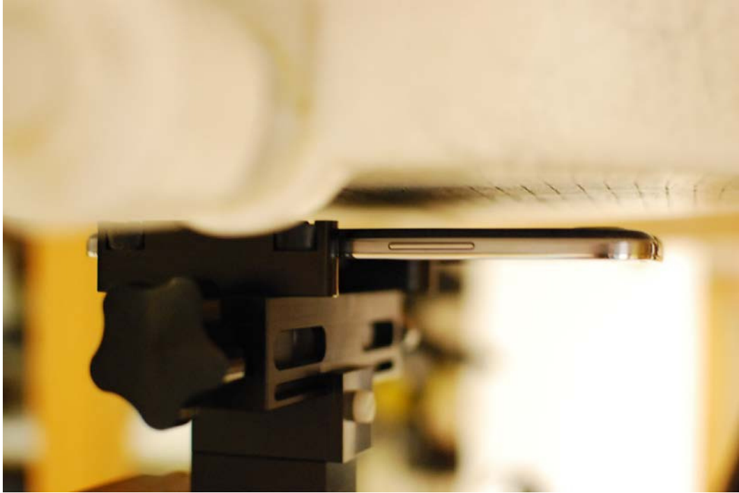
SAR Test Setup Photo 5: Back at 1.0 cm
