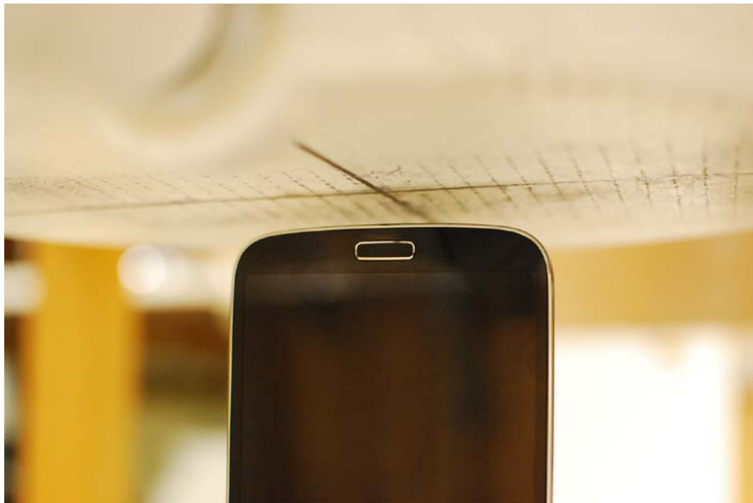
SAR Test Setup Photo 8: Bottom at 1.0 cm
