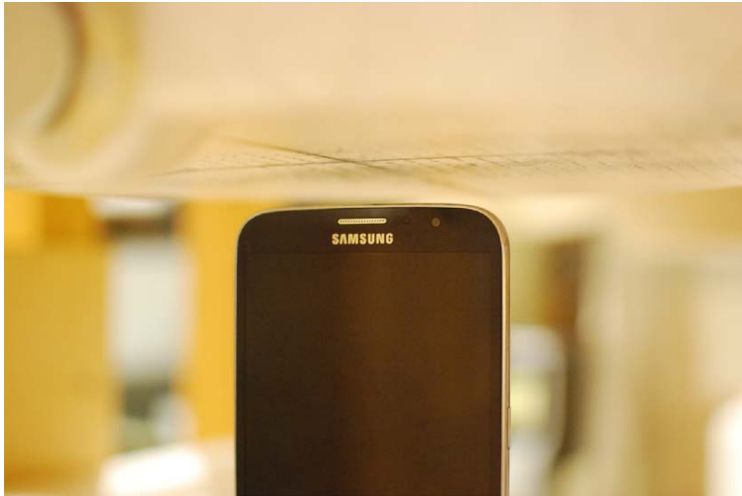
SAR Test Setup Photo 7: Top at 1.0 cm
