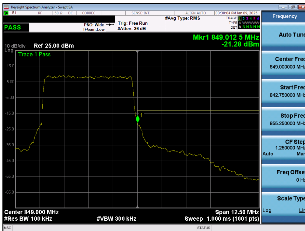
Plot 7-41. Upper Band Edge Plot (NR Band n5 – 5.0MHz - Full RB - Ant1)
