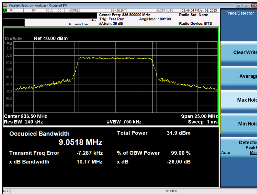
Plot 7-4. Occupied Bandwidth Plot (LTE Band 26/5 - 10MHz 16-QAM - Full RB - Ant1)
