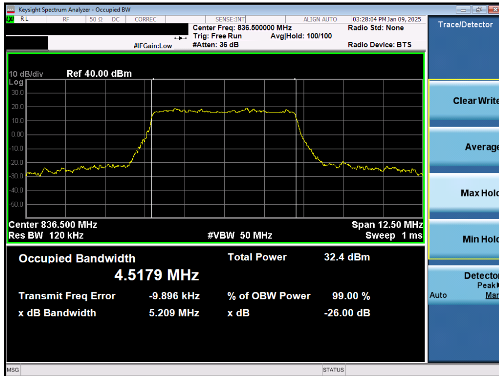
Plot 7-21. Occupied Bandwidth Plot (NR Band n5 - 5MHz QPSK - Full RB - Ant1)
