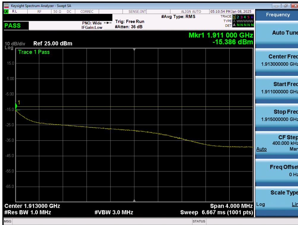
Plot 7-101. Extended Upper Band Edge Plot (WCDMA PCS – Ch. 9538 - Ant 2)
