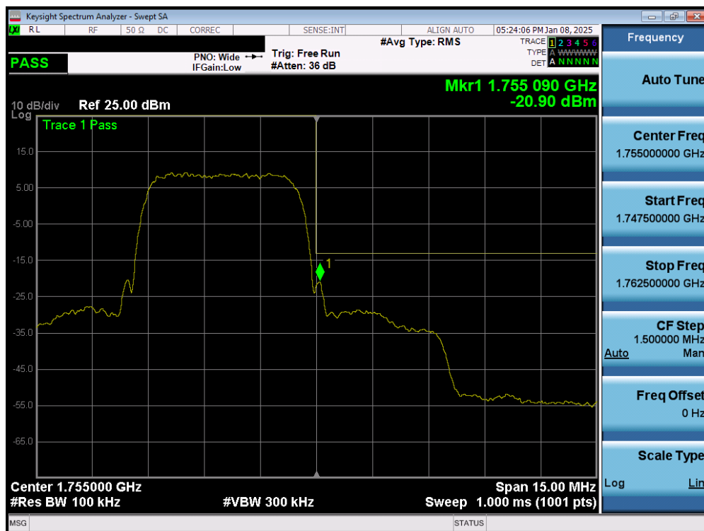
Plot 7-169. Upper Band Edge Plot (WCDMA AWS – Ch. 1513 – Ant2)
