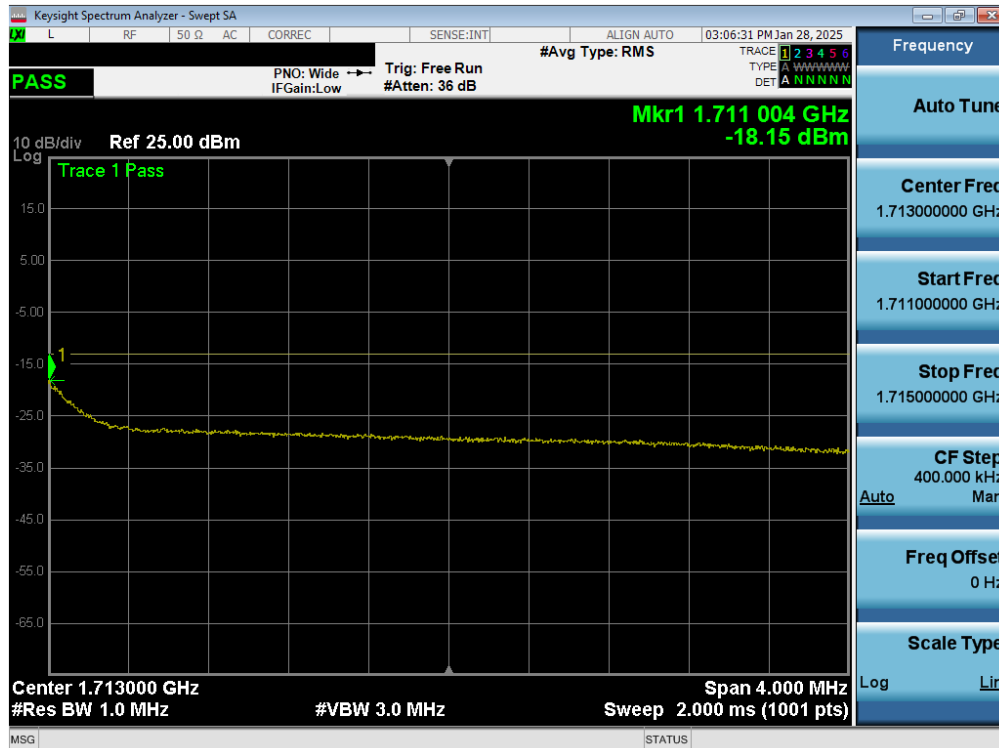
Plot 7-194. Upper Extended Band Edge Plot (NR Band n70 - 10.0MHz - Full RB - Ant4)
