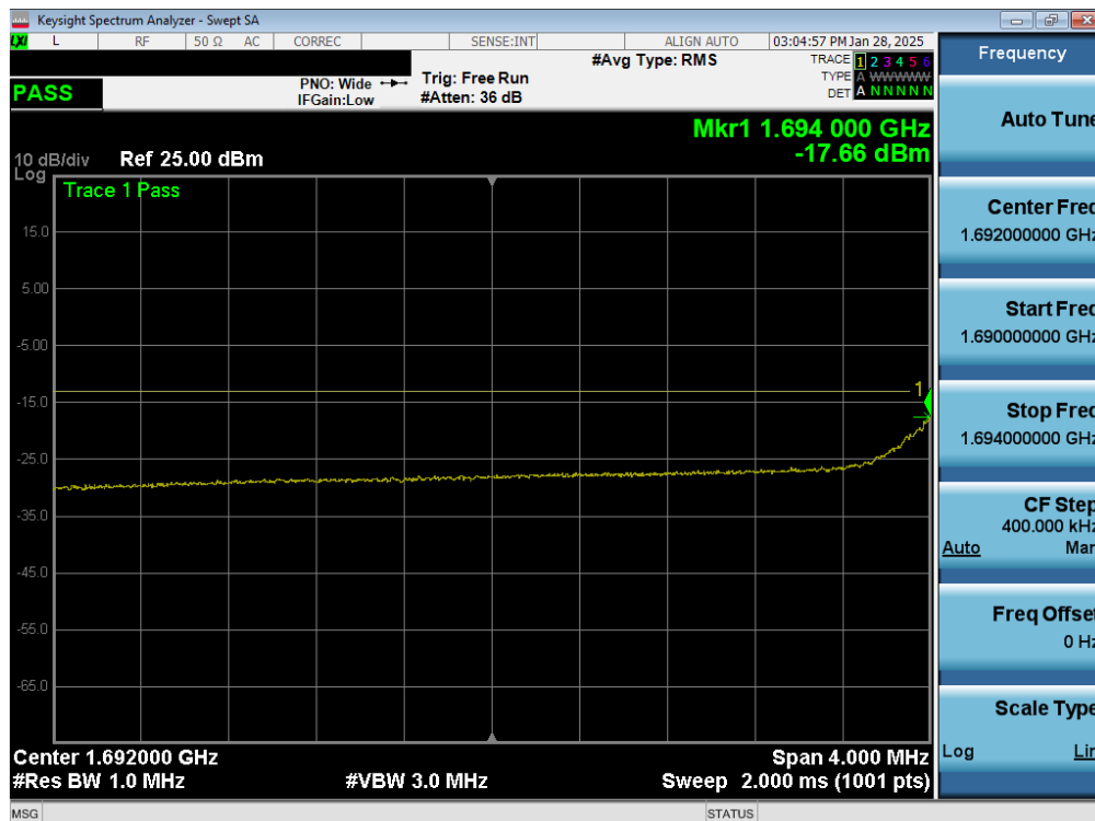
Plot 7-192. Lower Extended Band Edge Plot (NR Band n70 – 10.0MHz - Full RB – Ant4)
