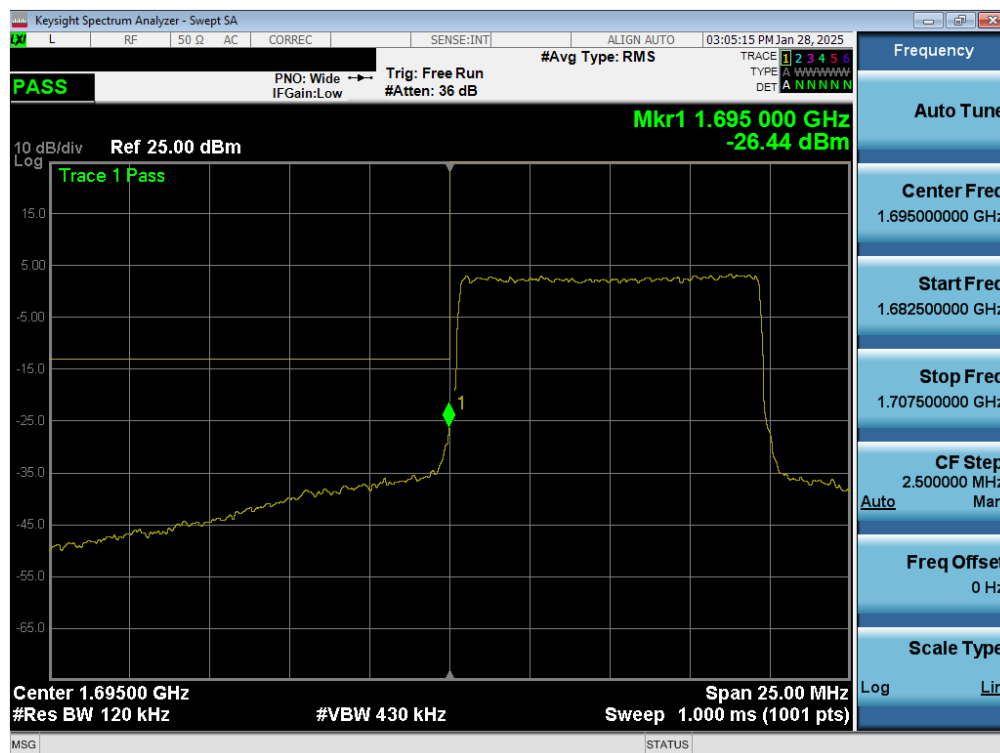
Plot 7-191. Lower Band Edge Plot (NR Band n70 – 10.0MHz - Full RB – Ant4)
