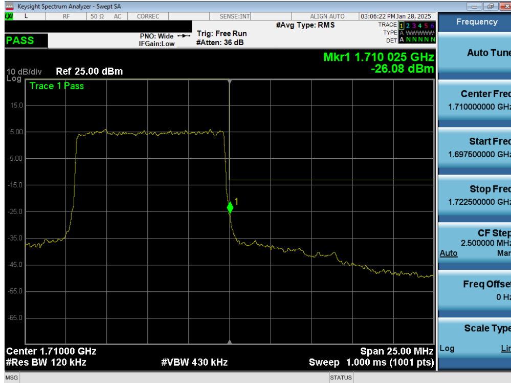
Plot 7-193. Upper Band Edge Plot (NR Band n70 - 10.0MHz - Full RB - Ant4)
