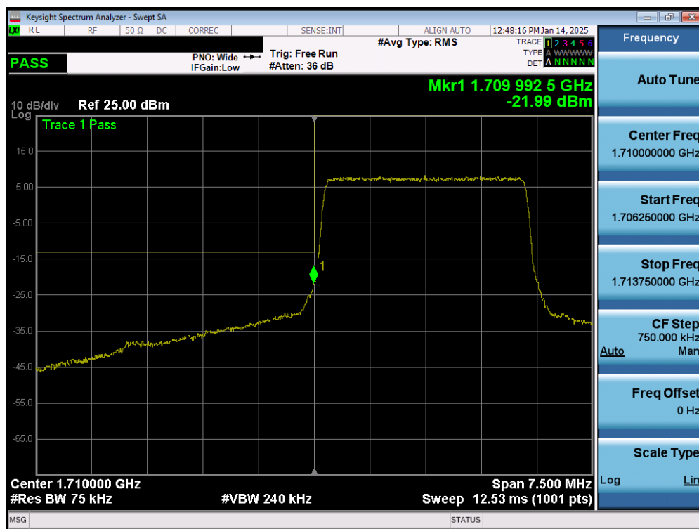
Plot 7-185. Lower Band Edge Plot (LTE Band 66/4 - 3MHz QPSK – Full RB – Ant4)
