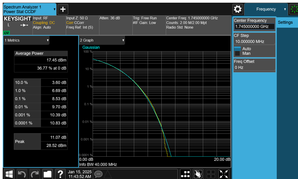
Plot 7-215. PAR Plot (NR Band n66 - 40.0MHz CP-OFDM 256-QAM - Full RB – Ant4)
