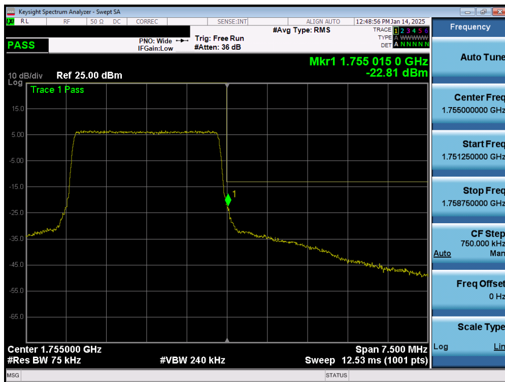
Plot 7-187. Upper Band Edge Plot (LTE Band 4 - 3MHz QPSK – Full RB – Ant4)
