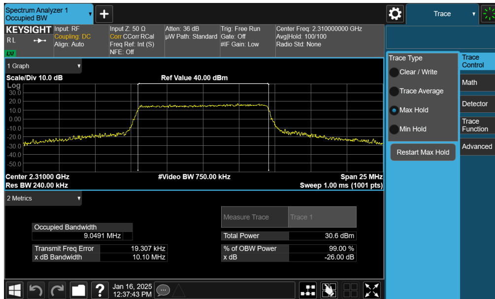
Plot 7-8. Occupied Bandwidth Plot (LTE Band 30 - 10MHz 16-QAM - Full RB - Ant 2)
