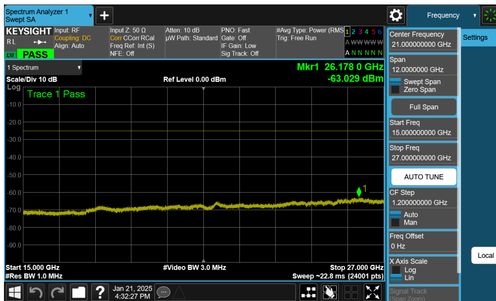
Plot 7-97. Conducted Spurious Plot (LTE Band 7 - 20MHz QPSK - RB Size 1, RB Offset 0 - Low Channel - Ant 2)
