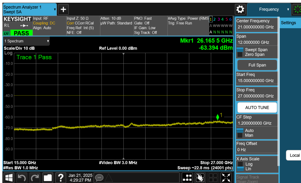
Plot 7-109. Conducted Spurious Plot (LTE Band 30 - 10MHz QPSK - RB Size 1, RB Offset 0 - Ant 4)
