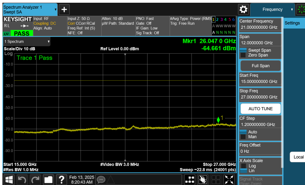
Plot 7-112. Conducted Spurious Plot (LTE Band 7 - 20MHz QPSK - RB Size 1, RB Offset 0 - High Channel - Ant 4)
