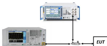
Figure 7-1. Test Instrument & Measurement Setup
