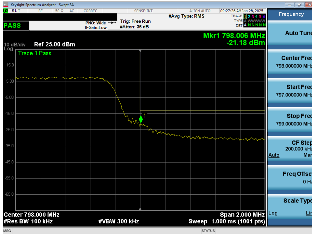
Plot 7-38. Upper Band Edge Plot (LTE Band 14, 5MHz QPSK - RB Size 50)
