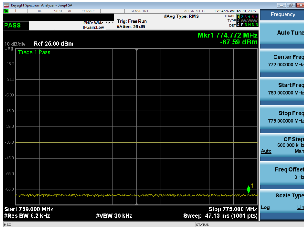
Plot 7-43. Lower Emission Mask Plot (NR Band n14 - 5MHz BPSK - Low Channel)
