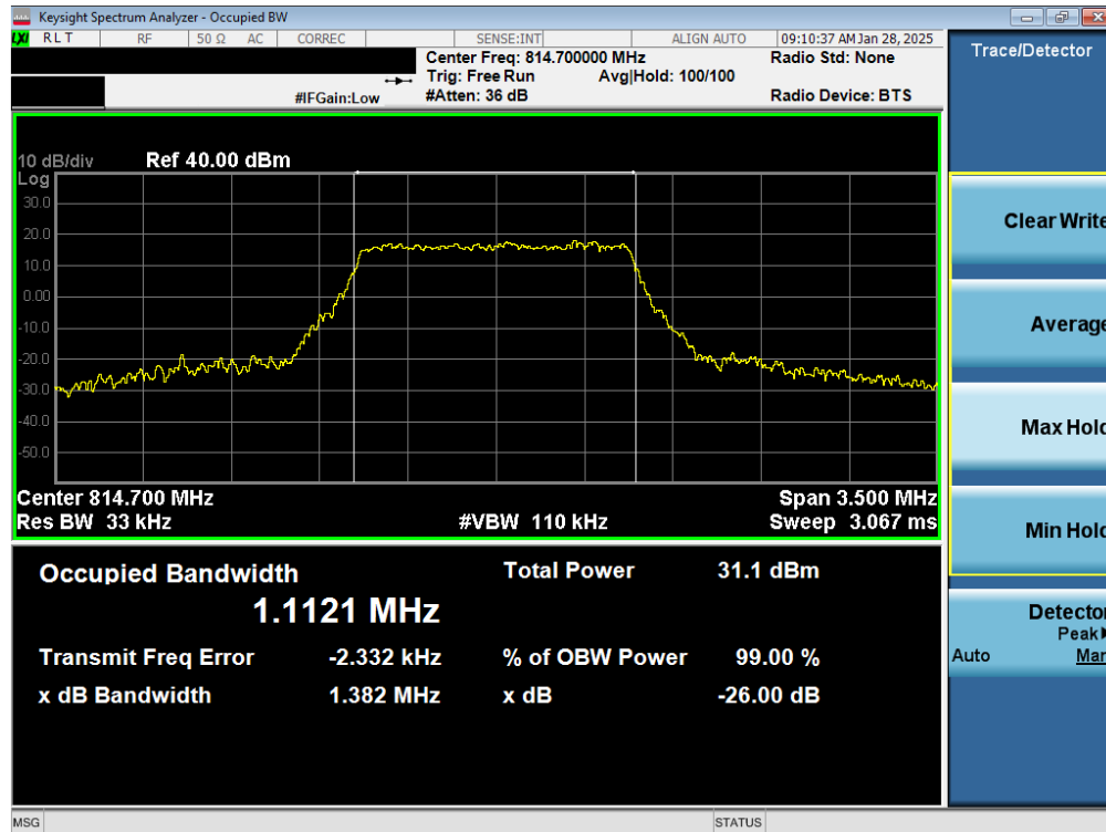
Plot 7-19. Occupied Bandwidth Plot (LTE Band 26 – 1.4MHz 16-QAM Low Channel - Full RB)
