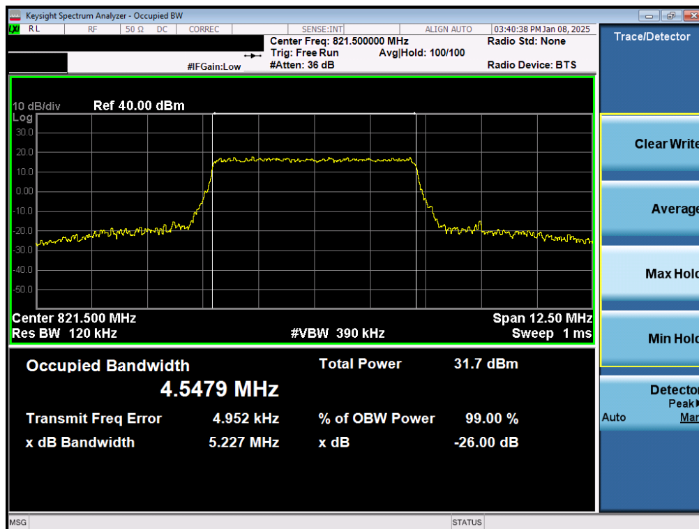
Plot 7-12. Occupied Bandwidth Plot (LTE Band 26 - 5MHz 16-QAM High Channel - Full RB)
