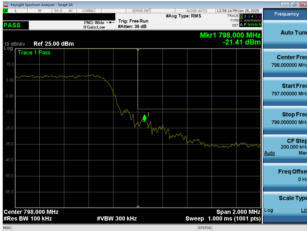
Plot 7-44. Channel Edge Plot (NR Band n14 - 5MHz BPSK - High Channel)
