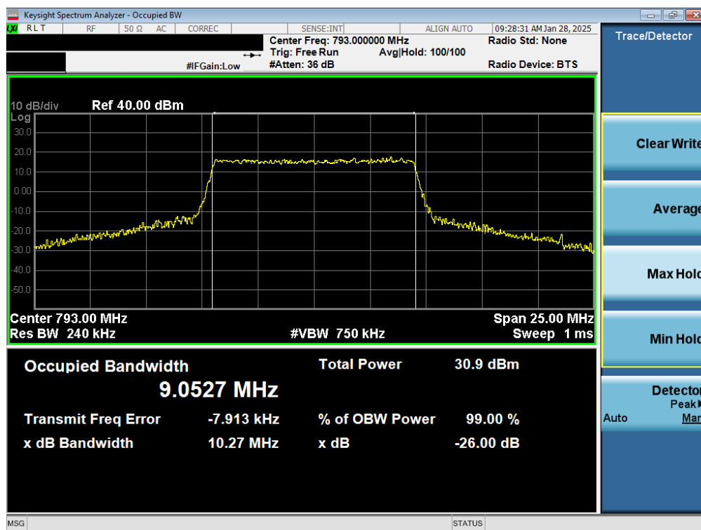
Plot 7-2. Occupied Bandwidth Plot (LTE Band 14 - 10MHz 16-QAM - Full RB)
