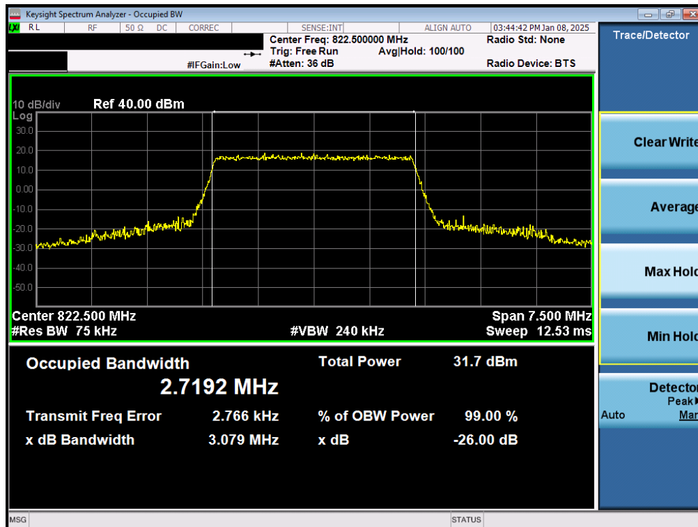
Plot 7-16. Occupied Bandwidth Plot (LTE Band 26 - 3MHz 16-QAM High Channel - Full RB)
