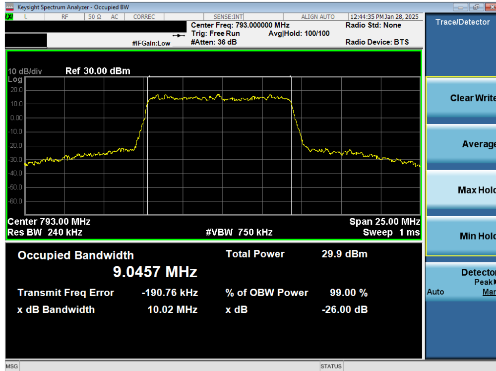
Plot 7-23. Occupied Bandwidth Plot (NR Band n14 - 10MHz 16-QAM - Full RB)
