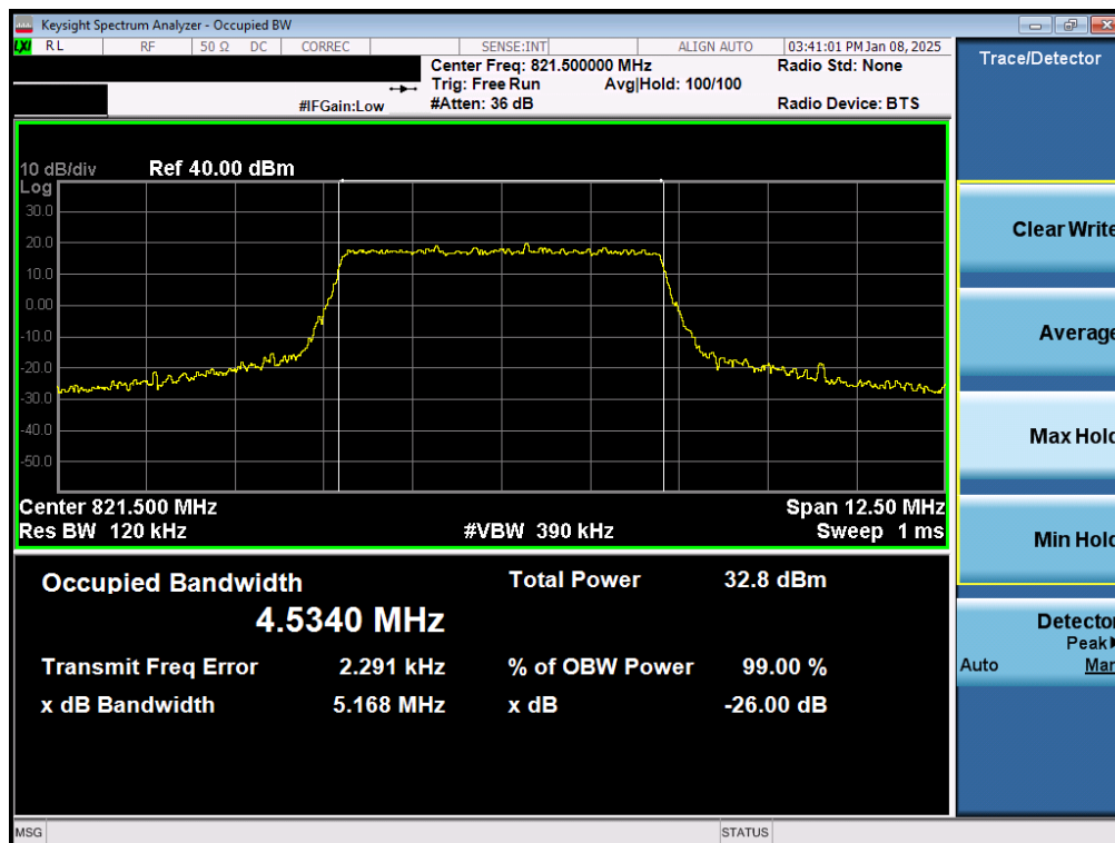
Plot 7-10. Occupied Bandwidth Plot (LTE Band 26 - 5MHz QPSK High Channel - Full RB)
