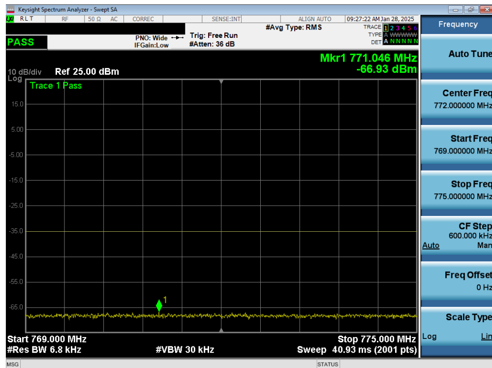
Plot 7-37. Lower Emission Mask Plot (LTE Band 14, 5MHz QPSK - RB Size 50)
