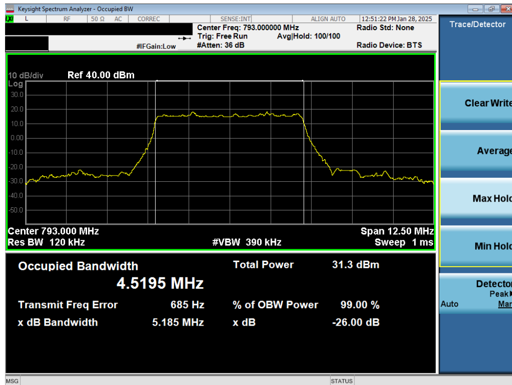
Plot 7-24. Occupied Bandwidth Plot (NR Band n14 - 5MHz \pi/2 BPSK - Full RB)
