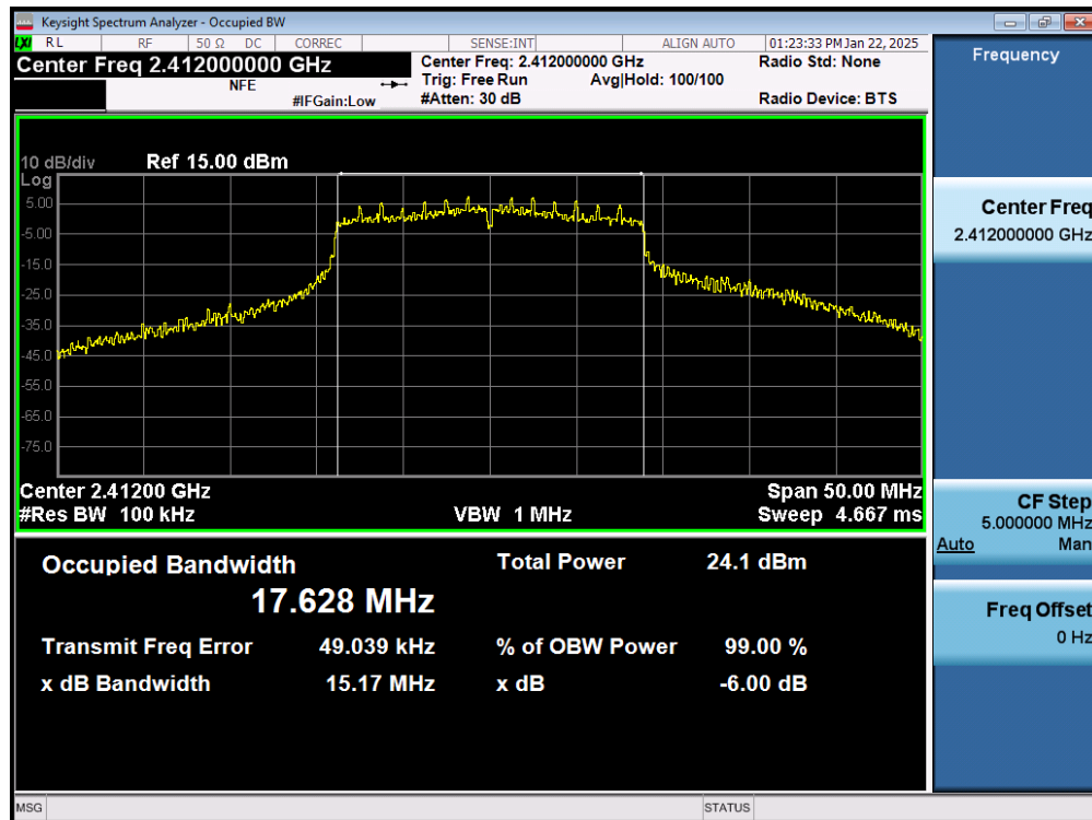
Plot 7-22. 6dB Bandwidth Plot (802.11n (2.4GHz) – Ch. 1) MIMO ANT2
