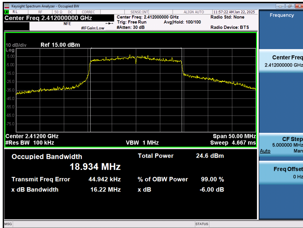
Plot 7-13. 6dB Bandwidth Plot (802.11ax (2.4GHz) – Ch. 1) MIMO ANT1
