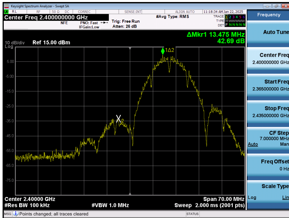
Plot 7-61. Band Edge Plot (802.11b – Ch. 1) MIMO ANT1
