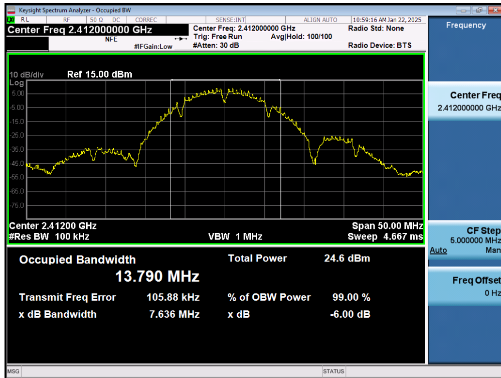
Plot 7-1. 6dB Bandwidth Plot (802.11b – Ch. 1) MIMO ANT1
