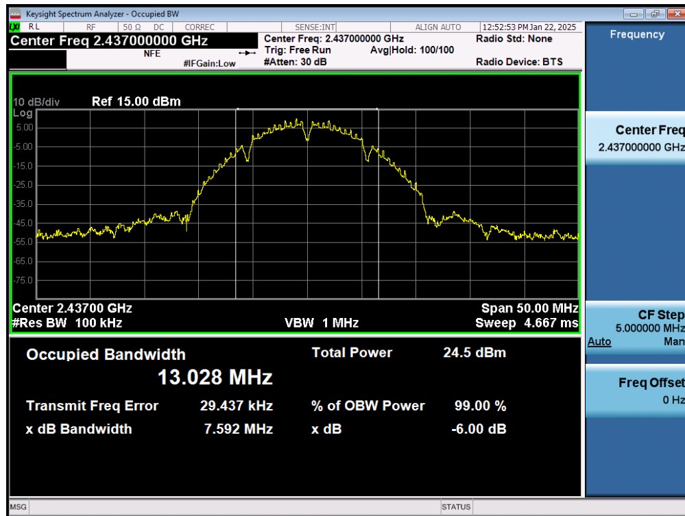
Plot 7-17. 6dB Bandwidth Plot (802.11b – Ch. 6) MIMO ANT2
