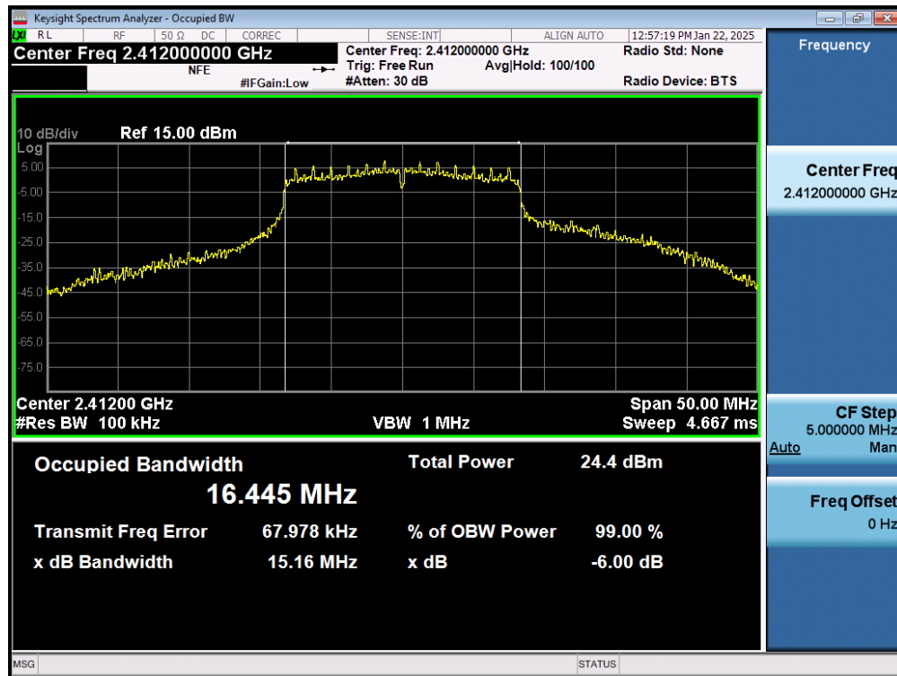
Plot 7-19. 6dB Bandwidth Plot (802.11g – Ch. 1) MIMO ANT2
