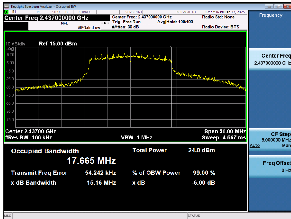
Plot 7-8. 6dB Bandwidth Plot (802.11n (2.4GHz) – Ch. 6) MIMO ANT1
