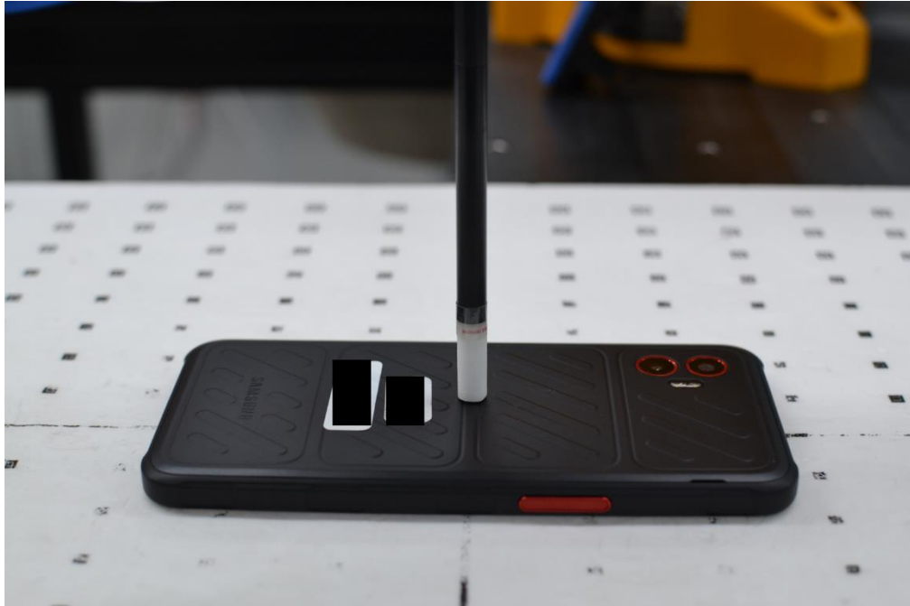
SAR Test Setup Photo 19 – PD, Back Side at 2mm
