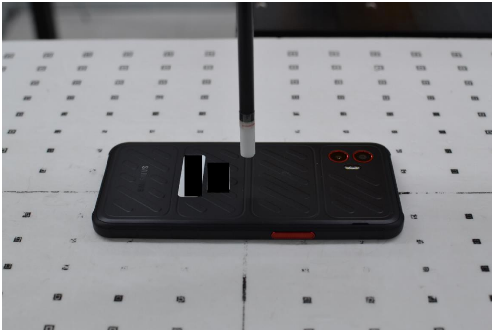
SAR Test Setup Photo 20 – PD, Back Side at 8.58mm
