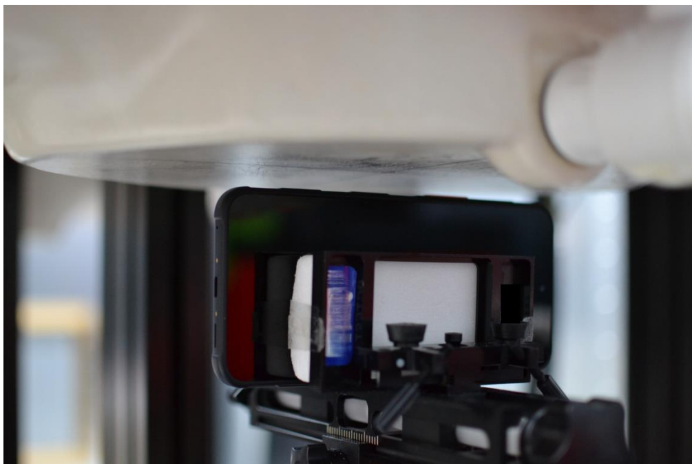
SAR Test Setup Photo 13 – Hotspot, Left Edge at 10mm
