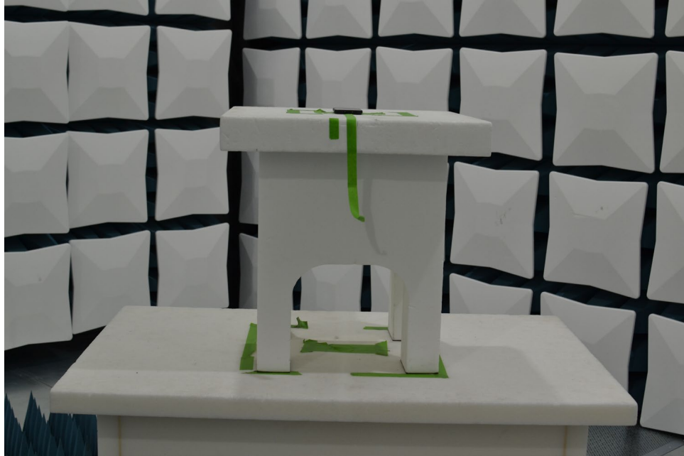
Figure 3. Test Setup – X Position – 1GHz-40GHz
