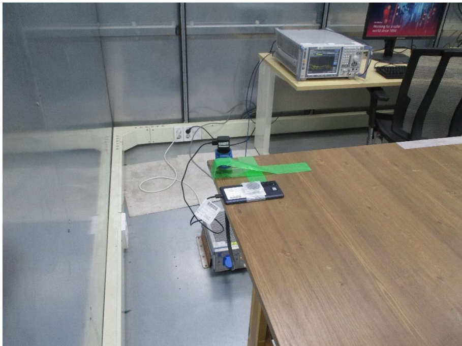
AC LINE CONDUCTED REAR TEST PHOTO(WPT)
