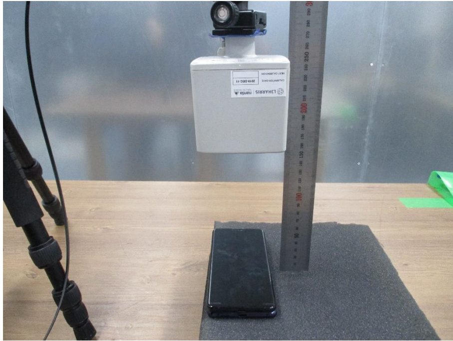
Top charger below client (20cm distance)
