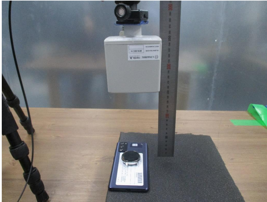
Top charger below client (20cm distance)
