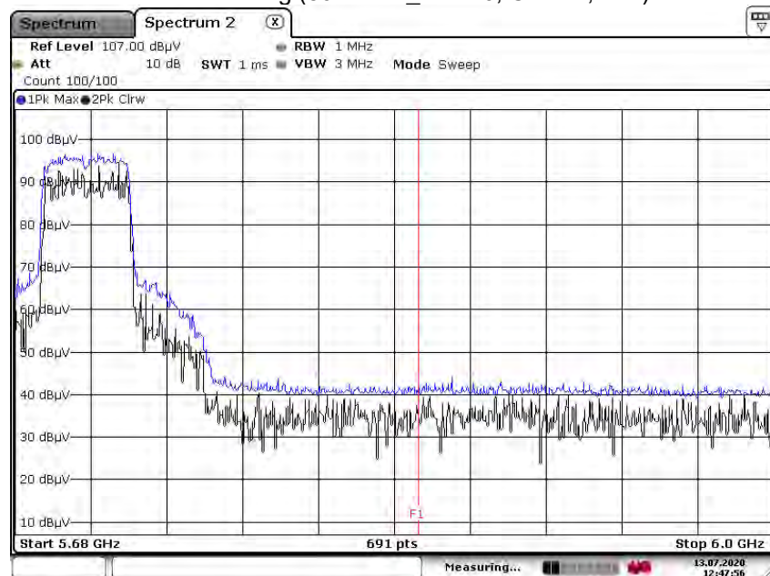
Peak Reading (802.11ac_VHT40, Ch.142, Z-H)
